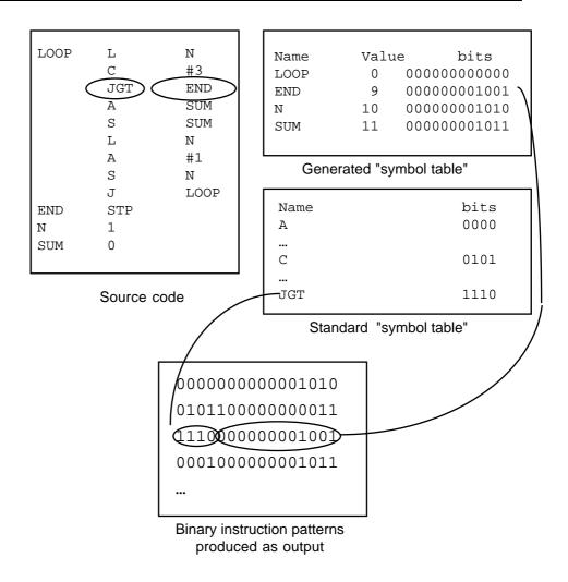
Figure 2.7 Generating code in "pass 2" of the assembly process
