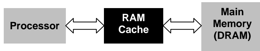
Figure 13-12 Cache Placement between Main Memory and Processor
