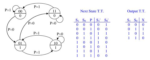
28. The three Boolean expressions below represent the *next state bits* ( $S_0'$  and  $S_1'$ ) and the *output bit* X based on the *current state* ( $S_0$  and  $S_1$ ) and the *input A*. Draw the logic circuit for the state machine including the latches and output circuitry. Be sure to label the latch inputs and other signals.
