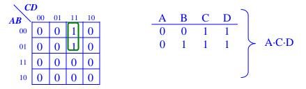
The resulting product has three inputs. You'll find that regardless of how the 2 cell rectangle is arranged, the resulting product will always have 3 inputs.
