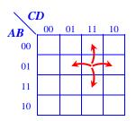
Since a square only has 4 sides, it can only represent 4 single-bit changes in the inputs. Therefore, 4 is the maximum.
