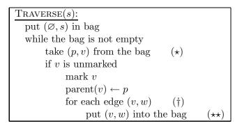
Notice that we're keeping *edges* in the bag instead of *vertices*. This is because we want to remember, whenever we visit a vertex v for the first time, which previously-visited vertex p put v into the bag. The vertex p is called the *parent* of v.
