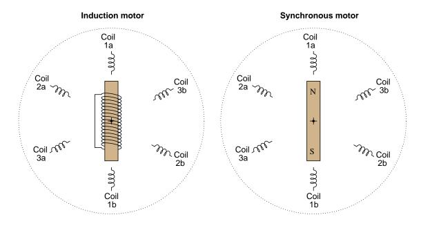
Synchronous AC motors use a permanent magnet rotor, while induction motors use an electromagnet rotor. Explain what practical difference this makes in each motor's operation, and also explain the meaning of the motors' names. Why is one called "synchronous" and the other called "induction"?
