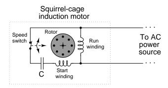
Explain why this special winding is necessary for the motor to start, and also why there is a capacitor connected in series with this start winding. What would happen if the start switch, capacitor, or start winding were to fail open?
