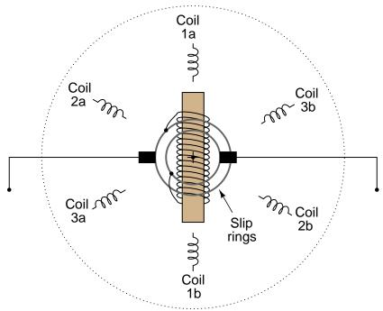
Explain how this motor can be operated as either a synchronous motor or a "plain" induction motor.  $\underline{\text{file }00741}$
