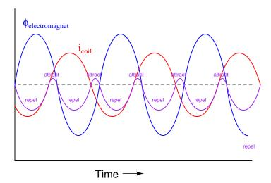
Given a phase shift between the two currents greater than 90 degrees (approaching 180 degrees), there is greater repulsion force for greater duration than there is attractive force. If the coil were a superconducting
