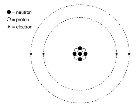
Neutrons reside in the center ("nucleus") of the atom, as do protons. Neutrons are electrically neutral (no charge), while protons have a positive electrical charge. Electrons, which reside outside the nucleus, have negative electrical charges.
