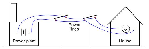
Why would anyone use two wires to conduct electricity from a power plant to a house, as shown, when they could simply use one wire and a pair of *ground* connections, like this?
