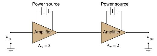
Also, convert the voltage gains of each amplifier into units of decibels, then convert the overall voltage gain ratio into units of decibels as well.
