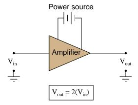
If we were to try to rate this amplifier's gain in terms of the relative power dissipated by a given load resistance ( $P_{load}$  when powered by  $V_{out}$ , versus  $P_{load}$  when powered by  $V_{in}$ ), what decibel figure would we calculate?
