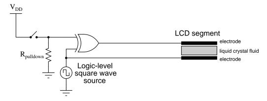
Consider the square wave voltage source in this schematic as a source of alternating "high" and "low" logic states, 5 volts and 0 volts respectively. Determine what sort of voltage exists across the liquid crystal fluid with the switch in the open position as well as the closed position, and from this determine which switch position results in a darkened LCD versus a transparent LCD.
