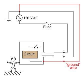
But why not eliminate all that extra wiring, and simply connect the third hole on the power receptacle to the "neutral" wire?
