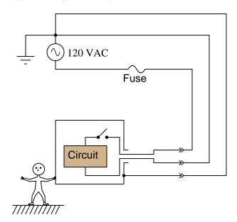
Explain how this grounding connection makes the appliance safer for any one touching its metal case.  $\underline{\rm file}~00315$
