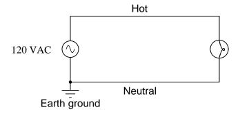
Follow-up question #1: in a power circuit such as this, there is typically a single fuse or circuit breaker for overcurrent protection. Identify the *best* location to place this fuse or circuit breaker in the circuit.
