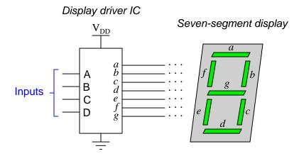
The behavior of the display driver IC may be represented by a truth table with seven outputs: one for each segment of the seven-segment display (a through g). In the following table, a "1" output represents an active display segment, while a "0" output represents an inactive segment:
