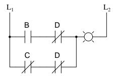
Follow-up question: although the relay circuit shown above does satisfy the minimal SOP Boolean expression, there is a way to make it simpler yet. Hint: done properly, you may eliminate one of the contacts in the circuit!
