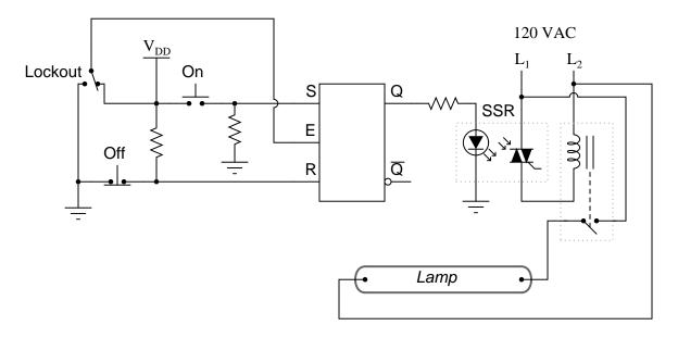
Based on your knowledge of how gated S-R latches function, what is the purpose of the "Lockout" switch? Also, explain how the CMOS latch is able to exert control over the high-power lamp (i.e. explain the operation of the interposing devices between the latch and the lamp).
