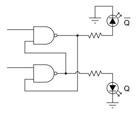
Identify which of the two input lines is the *Set*, and which is the *Reset*, and then write a truth table describing the function of this circuit.
