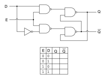
Complete the truth table for this D latch circuit, and identify which rows in the truth table represent the set, reset, and latch states, respectively.
