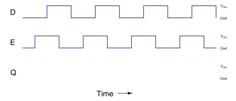
Then, determine the output of a D-type latch when the phase relationship is reversed, (D leading E by  $90^{\circ}$ , instead of E leading D by  $90^{\circ}$ ):
