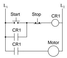
Draw the CMOS logic gate equivalent of this motor start-stop circuit, using these two pushbutton switches as inputs:
