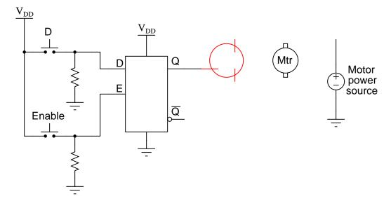
Also, comment on whether your MOSFET sources current to the motor or sinks current from the motor.
