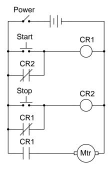
The circuit works fine, except that sometimes the motor starts all by itself when the circuit is first powered up! Other times, the motor remains off after power-up. In other words, the power-up state of this circuit is unpredictable.
