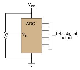
As the input voltage changes, the binary number output by the ADC will change as well. Suppose, though, that we want to have *sample-and-hold* capability added to this data acquisition circuit, to allow us to "freeze" the output of the ADC at will. Explain how using eight D latch circuits will give us this capability:
