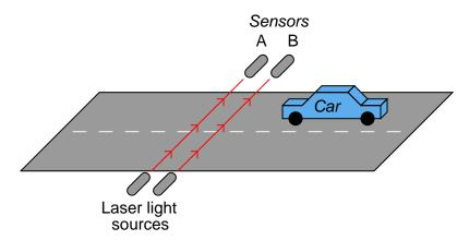
Both sensors connect to inputs on a D-type latch, which is then connected to some other circuitry to sound an alarm when a car goes down the road the wrong way:
