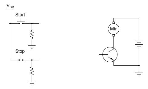
Make sure that your schematic is complete, showing how the logic gate will drive the electric motor (through the power transistor shown).
