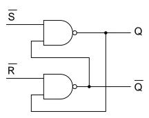
Add two more NAND gates to this circuit, converting it into a gated S-R latch, with an Enable (E) input, and write the truth table for the new circuit.
