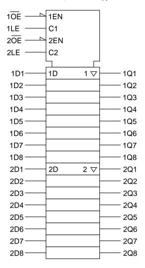
Note how the sixteen D latches are divided into two groups of eight. Explain the functions of the four inputs at the very top of the symbol (1EN, C1, 2EN, and C2). Which of these input lines correspond to the "Enable" inputs seen on single D-type latch circuits? Also, describe what the "wedge" shapes represent on the 1EN and 2EN input lines.
