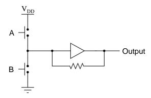
Why does the second buffer circuit need a resistor in the feedback loop?  $\underline{\text{file }02896}$
