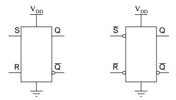
This simplifies schematic drawings where latches are used, much as the use of gate symbolism (as opposed to drawing individual transistors and resistors) simplifies the diagrams of more elementary digital circuits.
