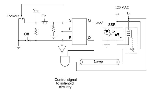
Follow-up question: there are better (safer) ways to accomplish this same function. For instance, suppose the TRIAC inside the SSR were to fail shorted, maintaining power to the lamp even when the latch goes into the "reset" mode. Would the door-lock logic shown here prevent someone from opening the door and getting exposed to the strong ultraviolet light? Explain your answer!
