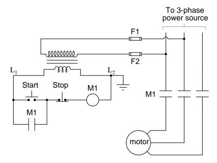
Explain the operation of this circuit, from the time the "Start" switch is actuated to the time the "Stop" switch is actuated. The normally-open M1 contact shown in the low-voltage control circuit is commonly called a seal-in contact. Explain what this contact does, and why it might be called a "seal-in" contact.
