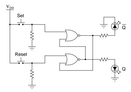
When the student powers up this circuit, she notices something strange. Sometimes the latch powers up in the *set* state (Q high and  $\overline{Q}$  low), and other times it powers up in the *reset* state (Q low and  $\overline{Q}$  high). The power-up state of their circuit seems to be unpredictable.
