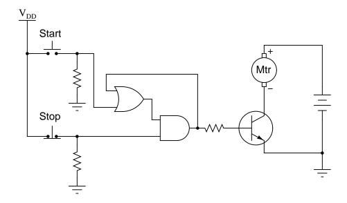
Follow-up question: why is the "Stop" switch always normally-closed in motor control circuits, whether it be relay logic or semiconductor logic? It is easy enough to invert a signal if we wish to, either by using a relay or by using a NOT gate, so shouldn't the choice of switch "normal" status be arbitrary?
