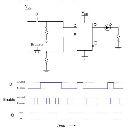
Complete the timing diagram, showing the state of the Q output over time as the input switches are actuated. Assume that Q begins in the low state on power-up:
