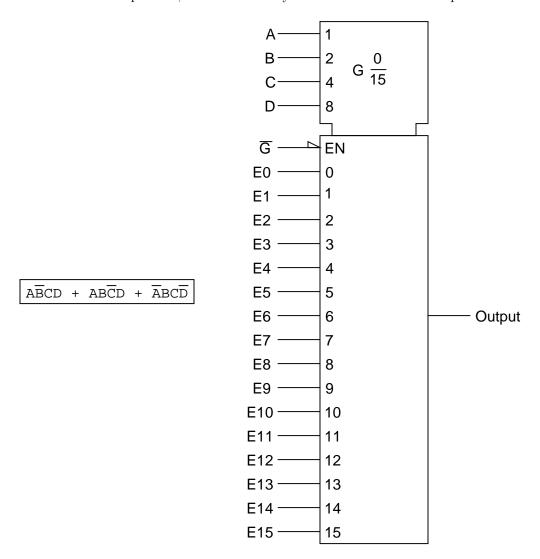
Show the wire connections necessary to make the multiplexer output the specified logic states in response to the data select (A, B, C, and D) inputs.
