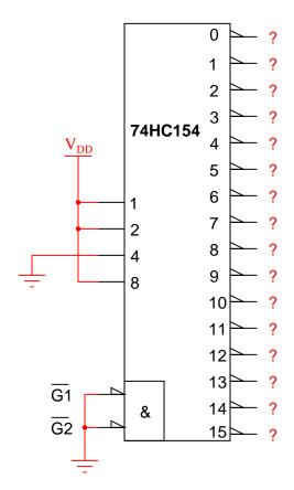
Identify the logic states of all output terminals given the input conditions shown.
