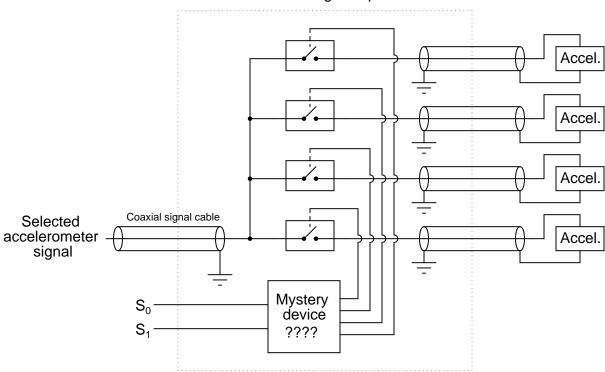
Identify the necessary "mystery device" shown in the schematic, which allows a binary input ( $S_0$  and  $S_1$  with four combinations of high/low states: 00, 01, 10, and 11) to activate just *one* bilateral switch at a time.
