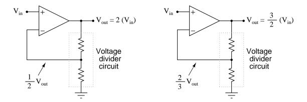
There is definitely a mathematical pattern at work in these noninverting opamp circuits: the overall voltage gain of the circuit is the *mathematical inverse* of the feedback network's voltage gain.
