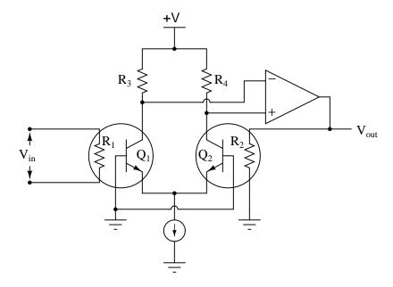
Describe how this circuit functions. What physical principle(s) does it use to derive an RMS value for  $V_{in}$ ? Why is it important that all identical components (transistors, resistors) be precisely matched?  $\frac{\text{file }01014}{\text{file }01014}$
