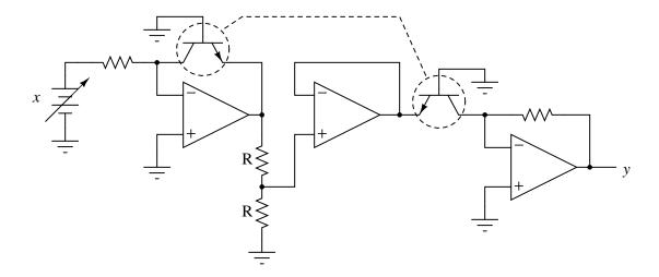
Challenge question: is there a part we could order that contains two matched, heat-stabilized transistors for an application such as this? Are there any other circuit applications you can think of that could benefit from using a precision-matched pair of transistors?
