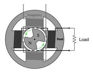
Like the first coil (the *real* coil), the imaginary coil's output voltage will also be sinusoidal. However, it will generate an output voltage at a different phase than the real coil's output voltage.
