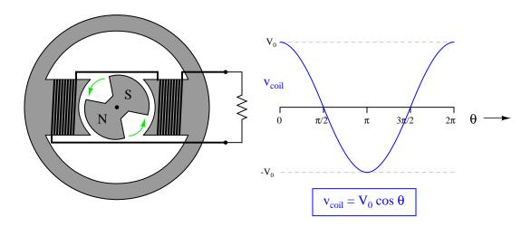
We may represent the coil's voltage with the equation  $v_{coil} = V_0 \cos \Theta$ . If we precisely know the peak voltage value  $(V_0)$  and the shaft position  $(\Theta)$ , we may precisely predict the coil voltage at any instant in time  $(v_{coil})$ .
