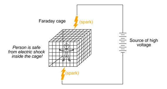
Explain how the principle of electrically common points protects the person inside the Faraday cage from being shocked by the outside source of high voltage. Discuss how this principle might apply to metal-frame automobiles and aircraft.
