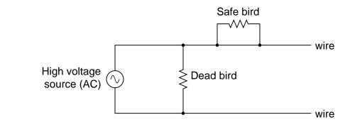
Determine whether or not a shock hazard exists for a person standing on the ground, by touching any one of the points labeled in this circuit:
