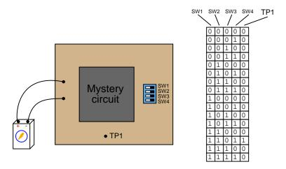
Based on this truth table "description" of the circuit, write an appropriate Boolean expression for this circuit.
