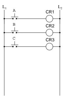
Implement the SOP logic function using contacts of relays CR1, CR2, and CR3. A partial ladder logic diagram has been provided for you.
