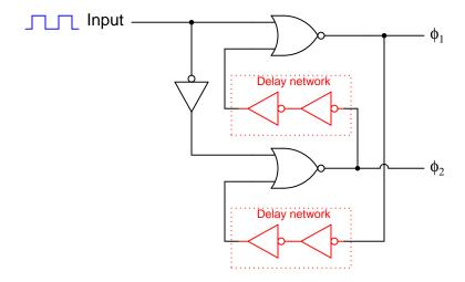
Assume that the only gates possessing propagation delays are the double-NOT gates (inside the dotted boxes), whose sole purpose it is to provide a short time delay in the feedback signals. Draw a timing diagram showing the two-phase clock signals ( $\phi_1$  and  $\phi_2$ ) in relation to the input clock waveform, and be prepared to explain how and why this circuit works:
