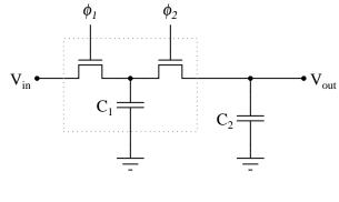
$$f_{-3dB} = \frac{f_{switch}C_1}{2\pi C_2}$$
