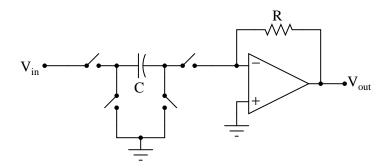
Research the resistance equivalence equations for each of these switched-capacitor networks (using N-channel MOSFETs as switches), describing the emulated resistance (R) as a function of switching frequency (f) and capacitance (C):
