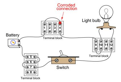
Taking voltage measurements with a voltmeter, how do you think this corrosion problem will reveal itself with the switch on the ON position? In other words, which voltage measurement in this circuit (i.e. between which pair or pairs of terminal block points) will be unusual as a result of the bad connection at point #4, and approximately how much voltage should that measurement be?
