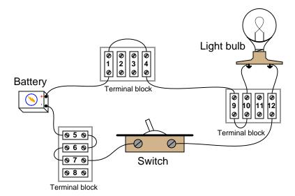
Determine whether or not voltage should be present between the following pairs of terminal block points with the switch in the ON position:
