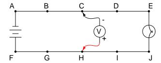
Using a voltmeter, a technician measures 0 volts between the points C and H. What does this single measurement indicate about the condition of the circuit? Be as specific as you can.
