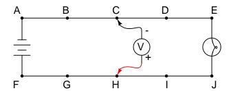
Using a voltmeter, a technician measures 0 volts between the points C and H. The result of this single measurement indicates which half of the circuit there is a definite problem in. What would you recommend as the *next* voltmeter measurement to take in troubleshooting the circuit, following the same "divide in half" strategy?
