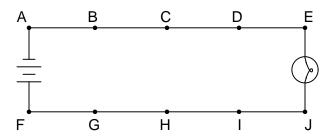
In this circuit, where would you *not* expect to measure significant voltage (between what pairs of test points)?
