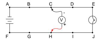
Using a voltmeter, a technician measures full battery voltage between the points C and H. What does this single measurement indicate about the condition of the circuit? Be as specific as you can.
