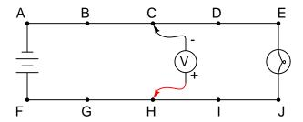
Using a voltmeter, a technician measures full battery voltage between the points C and H. The result of this single measurement indicates which half of the circuit there is a definite problem in. What would you recommend as the *next* voltmeter measurement to take in troubleshooting the circuit, following the same "divide in half" strategy?
