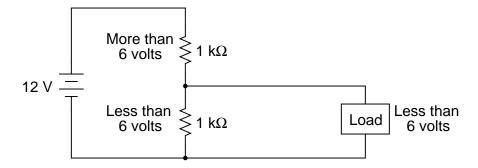
(Of course, with no load connected, the voltage across the lower resistor would be precisely 6 volts. With the load connected, the parallel combination of load and 1 k $\Omega$  resistor results in an effective resistance of less than 1 k $\Omega$  on the lower half of the divider, resulting in a voltage of less than half the total supply voltage.)
