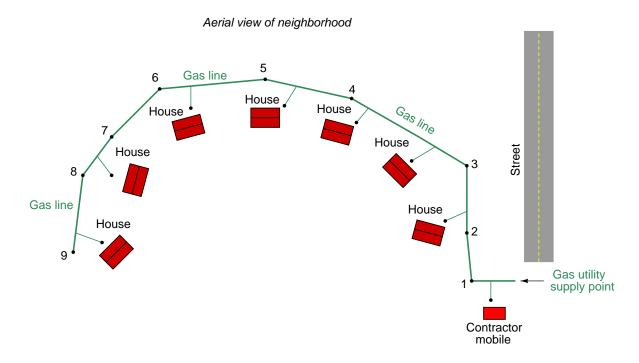
Each black dot on the diagram is a shutoff valve, used for isolating different sections of the service pipeline. Based on the heating technician's report, you conclude that the service pipeline going up to that house must not be "live," and that one of the numbered valves was probably left in the *off* position. But which one could it be?
