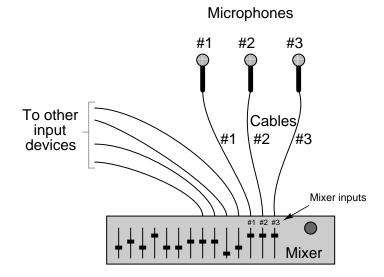
The purpose of the mixer is to function as a multi-channel audio signal amplifier, to control the volume of each sound channel so that a good "mix" is obtained for recording. The studio engineer will use the individual controls on the mixer to "blend" the inputs for the best recording tone and quality.
