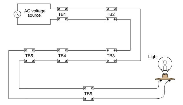
As you can see in the diagram, there are several terminal blocks ("TB") through which electrical power is routed to the light bulb. These terminal blocks provide convenient connection points to join wires together, enabling sections of wire to be removed and replaced if necessary, without removing and replacing *all* the wiring.
