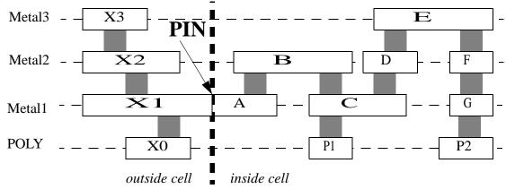
When the Metal2 segment "X2" is manufactured, the transistor area "P1" is exposed to antenna. When the Metal3 segment "X3" is manufactured, the transistor areas "P1" and "P2" are exposed to antenna. The smaller the exposed transistor area, the greater the damage. Therefore, using the area "P1" is pessimistic, using the area "P1+P2" is not safe.
