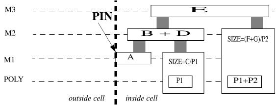
In order to describe this abstraction in ALF, the TARGET annotation within the context of SIZE is proposed. The value of the TARGET annotation is a PATTERN, corresponding to the transistor area exposed to antenna.
