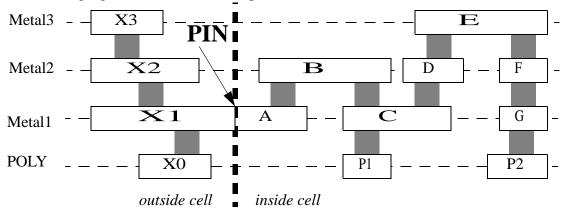
When the Metal2 segment "X2" is manufactured, the transistor area "P1" is exposed to antenna. When the Metal3 segment "X3" is manufactured, the transistor areas "P1" and "P2" are exposed to antenna. The smaller the exposed transistor area, the greater the damage. Therefore, using the area "P1" is pessimistic, using the area "P1+P2" is not safe.
