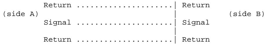
The return path must include all pins that are power or ground. In a loop inductance matrix, the diagonal terms represent the loop inductance of a specific conductor given a specific return path.
