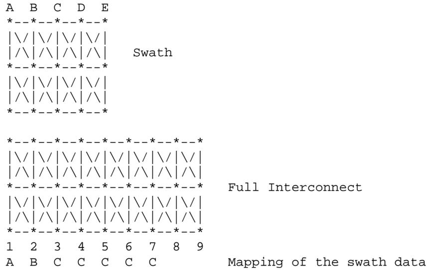
Starting at the center of the swath, the coupling pattern of just the center of the swath (column C in this example) is copied into the full interconnect matrix being constructed by the EDA tool. In this case, the data for the conductors in column C, lacking edge effects, may be used to represent several conductors near the center of the expanded matrix.
