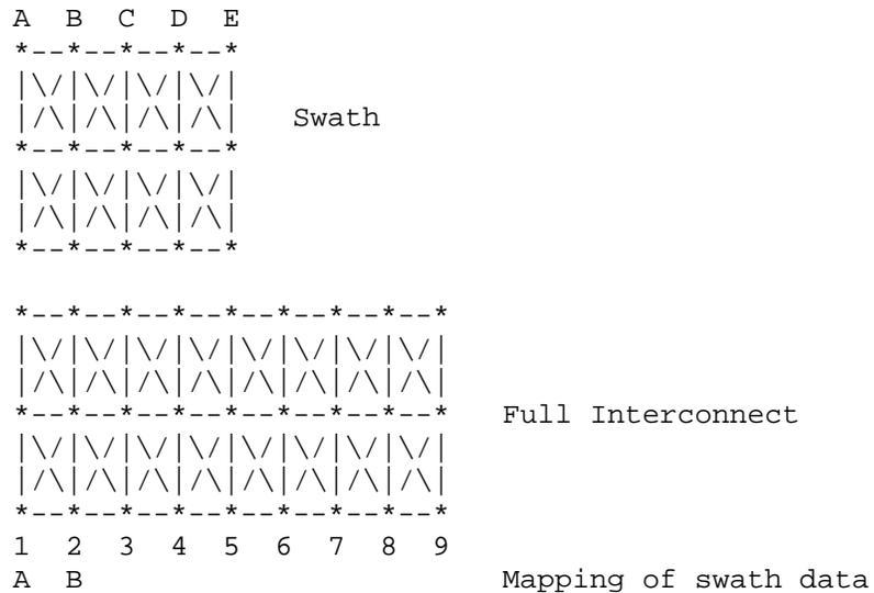
In this case, columns A and B of the swath data become columns 1 and 2 of the expanded interconnect.
