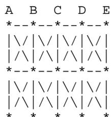
Notice that columns B, C, and D have the maximum amount of coupling to conductors on each side. However, columns A and E are only coupled to conductors on one sides.
