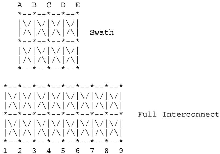
Centering is a way to map the swath matrix pins directly into the corresponding pins of the actual interconnect. For example, the swath above is centered about column 4 of the full sized interconnect. The paths of interest, including those of columns 3 and 5, are also described by swath matrix data that has coupling from both sides. However, because of edge effects, columns 2 and 6 are less accurately approximated by the corresponding swath columns (A & E, respectively).
