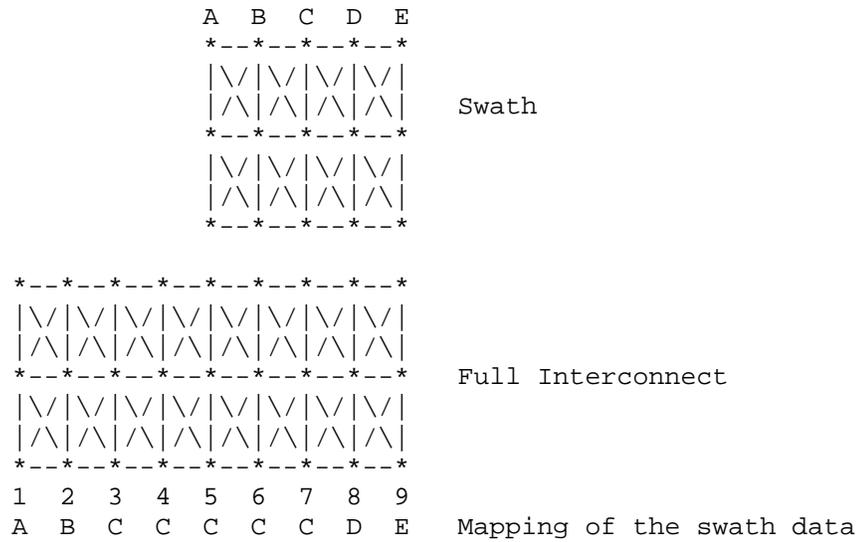
The final step is similar to step (a) above, but applied using the right side of the swath. When the swath is positioned against the right edge of the full interconnect as shown, the data for the rightmost
