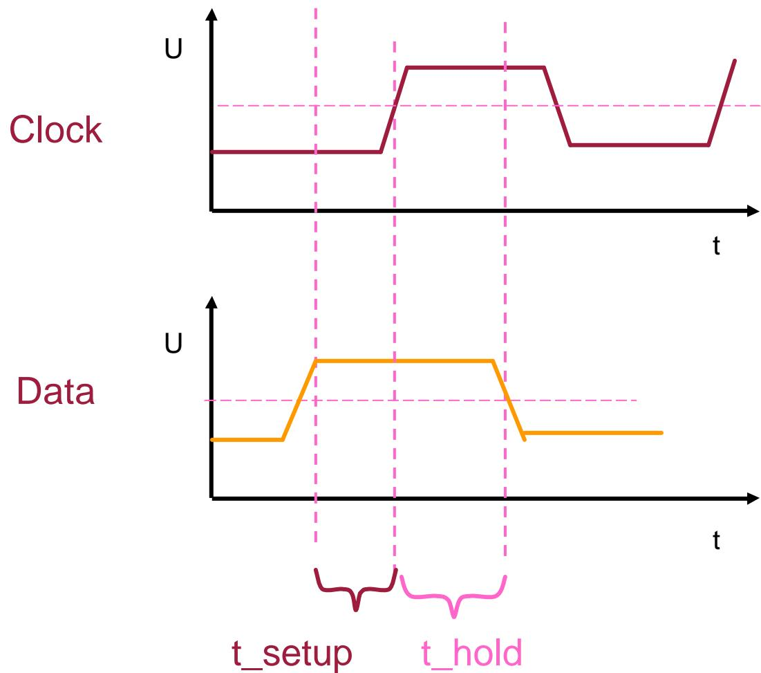
**$t_{\text{setup}}$ :** the time, the data has to be stable high, until the clk starts rising
