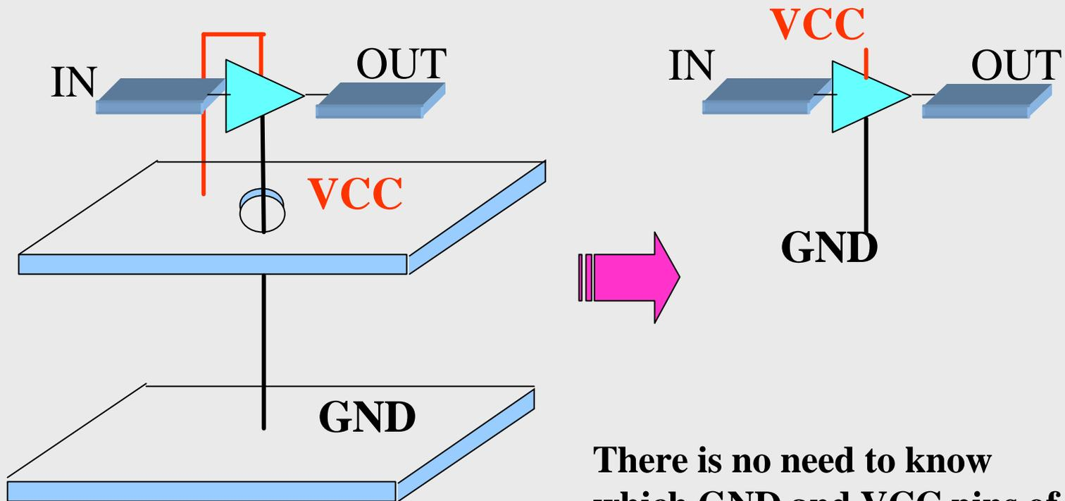
**There is no need to know which GND and VCC pins of package drivers and receivers are connected to**
