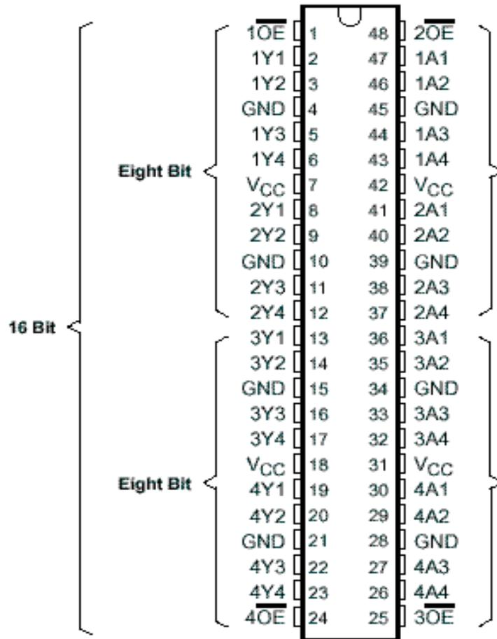
Many VCC and GND pins. Probably all VCC connected together inside IC. Same for Gnd. If we are simulating drivers on this IC, we connect their VCC to all VCC pads of this package on the PCB.
