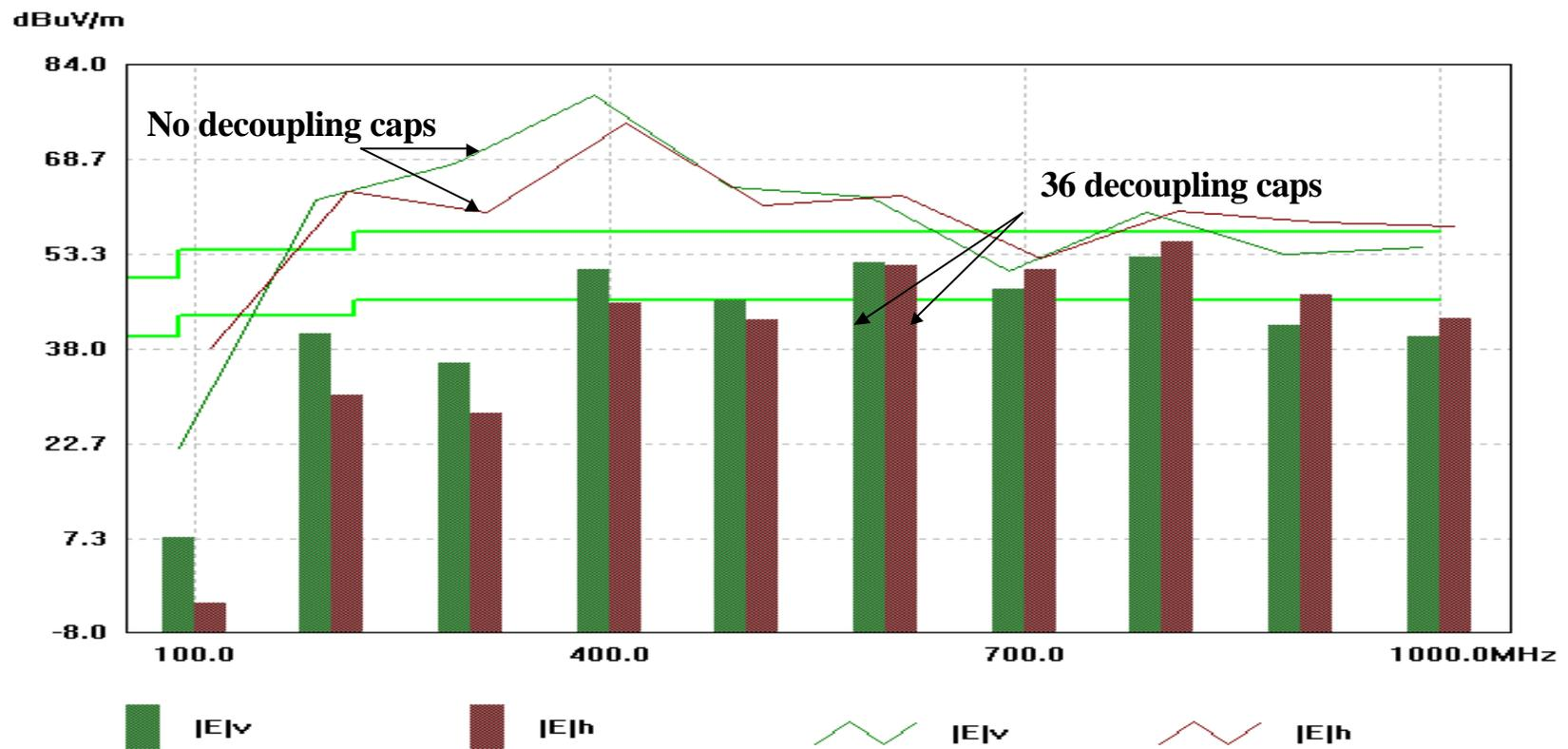
Edge radiation was calculated corresponding to waveforms in the previous slides. The higher power-ground noise without decoupling caps leads to much higher edge radiation. This was measured at a horizontal distance of 3m and a vertical distance of 3m from the board
