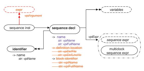
1) The **vpiArgument** iterator shall return the sequence instance arguments in the order that the formals for the sequence are declared, so that the correspondence between each argument and its respective formal can be made. If a formal has a default value, that value shall appear as the argument should the instantiation not provide a value for that argument.
