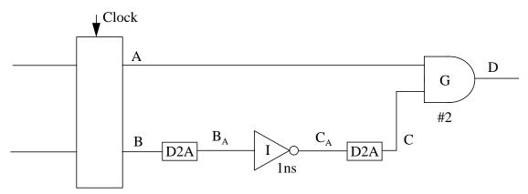
For the sake of argument we will assume the signal B is converted to  $B_A$  signal at  $C_A$  is converted to C with no timing errors, but the delay from  $B_A$  to  $C_A$  is only approximately 1nS so the signal C is handled in its own delta cycle. The evaluation of G to generate D occurs during that delta, but scheduling D requires rounding to the digital clock.
