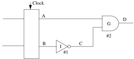
The inverter (I) has a one unit delay and the gate (G) has a two unit delay, so the digital delay from the clock edge to a result at D is three units (3ns). If the inverter is replaced with an analog equivalent the delay from the clock edge to D should still be three units:
