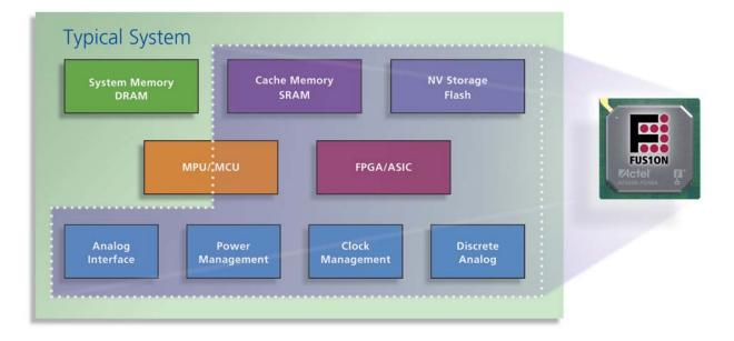
Actel Fusion integrates Flash memory, basic analog functionality, "scratch pad" SRAM, and programmable logic into the world's first monolithic mixed-signal FPGA. Embedding a soft microcontroller in the FPGA fabric turns Fusion into the ultimate programmable system chip.
