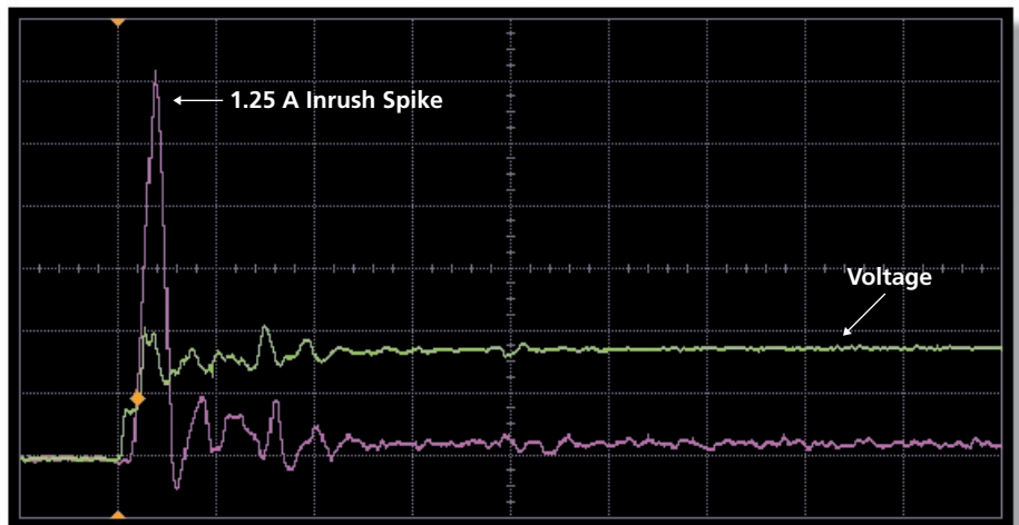
Figure 2: Actual SRAM FPGA Inrush Current
