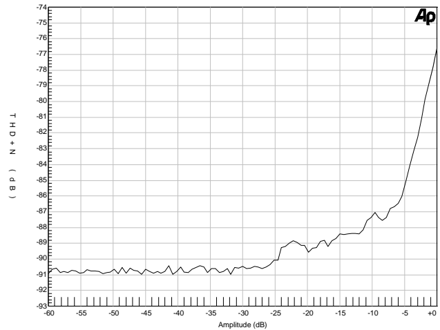
Figure 17. Headphone Output - THD+N versus Amplitude at 3.0 V
