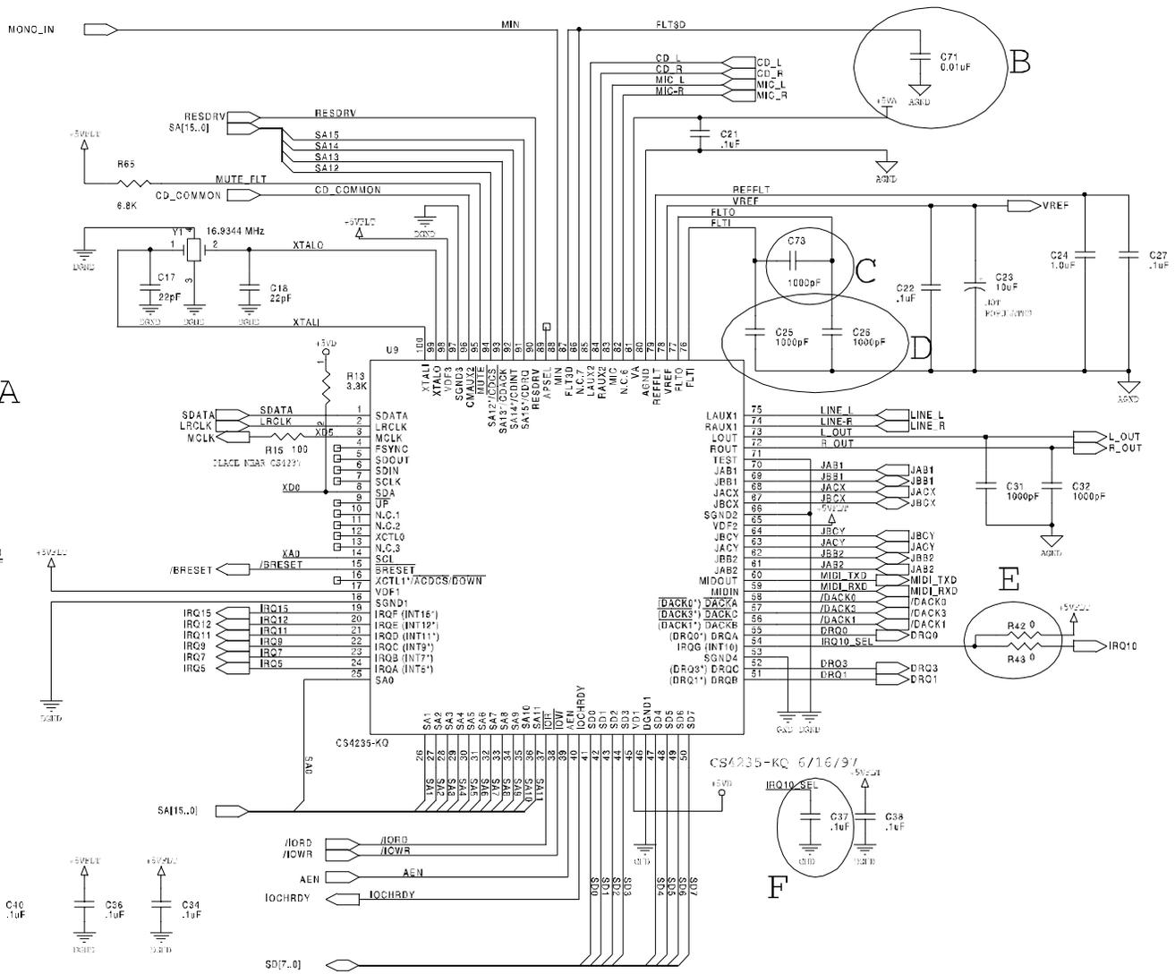
Figure 1. CS423xB to CS4235 Differences
