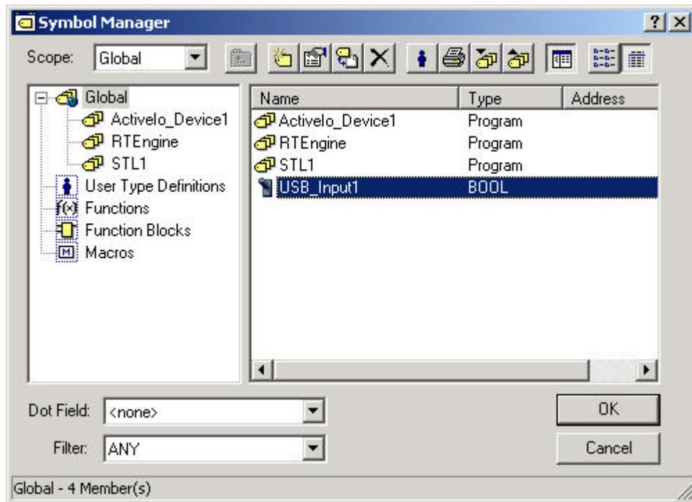
Select “Global” and “USB\_Input1” then click “OK” to continue. This process must be repeated to insert the “ReadBit” command. Once again select the “Insert” menu and choose “Symbol”. Be sure to select “ActiveIo\_Device1” and “ReadBit”. The dialog should appear as below:
