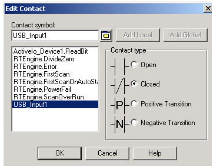
Select “USB\_Input1” and be sure the contact type is “Closed”. In our example we are using a closed contact because the example is done with one of our USB TTL digital I/O cards. With no input connected, the pull-up resistor on the input biases the input to a logical 1. When the input is connected, it is actually switched to ground. The closed contact is used as a means of inverting the input. Click “OK” to continue. The main screen should now appear as below:
