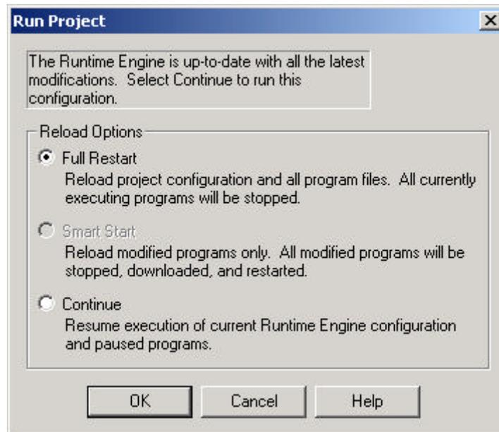
Be sure "Full Restart" is selected and click "OK". After the project loads, change the state of the input and watch the contact in the RLL program. When the input is true the contact should be green.
