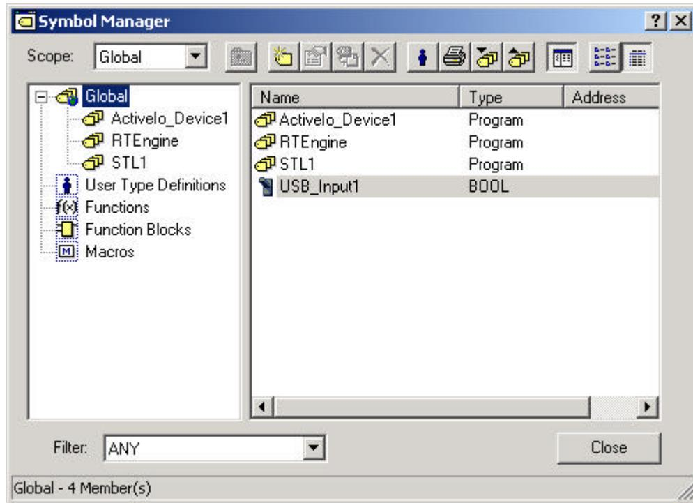
Click the “Close” button to complete adding this symbol. We will now use this symbol in conjunction with our ActiveIO “ReadBit” command to read the status of one input. The symbol and command must be inserted into the STL program. Click the “Insert” menu and select “Symbol” and a familiar dialog now appears:
