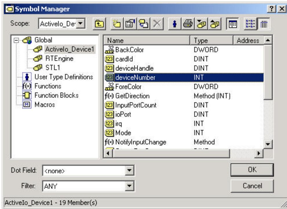
This will insert the ActiveIO “deviceNumber” command into your STL program. To complete this instruction you must assign your SeaIO device number to this command. After doing so the main screen should now look like this:
