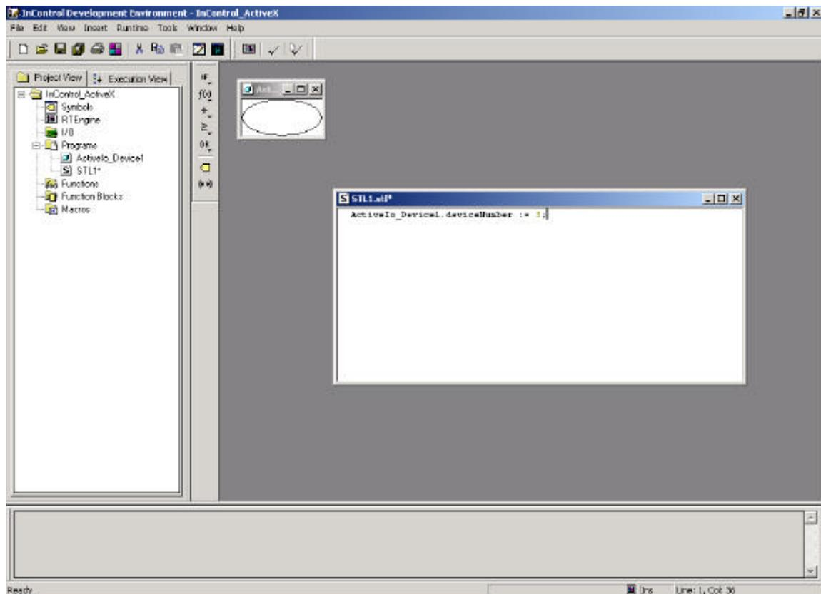
This command is used to open the card for access. In this example our SeaIO device number is 5. Your device number can be determined by using Device Manager to look at the installed SeaIO Devices. This will be shown in parenthesis as a card number (Card X). The next step is to create a Global symbol that can be used to return the status of one input bit. Start by clicking the “Tools” menu and selecting “Symbol Manager”. The following dialog should now be active:
