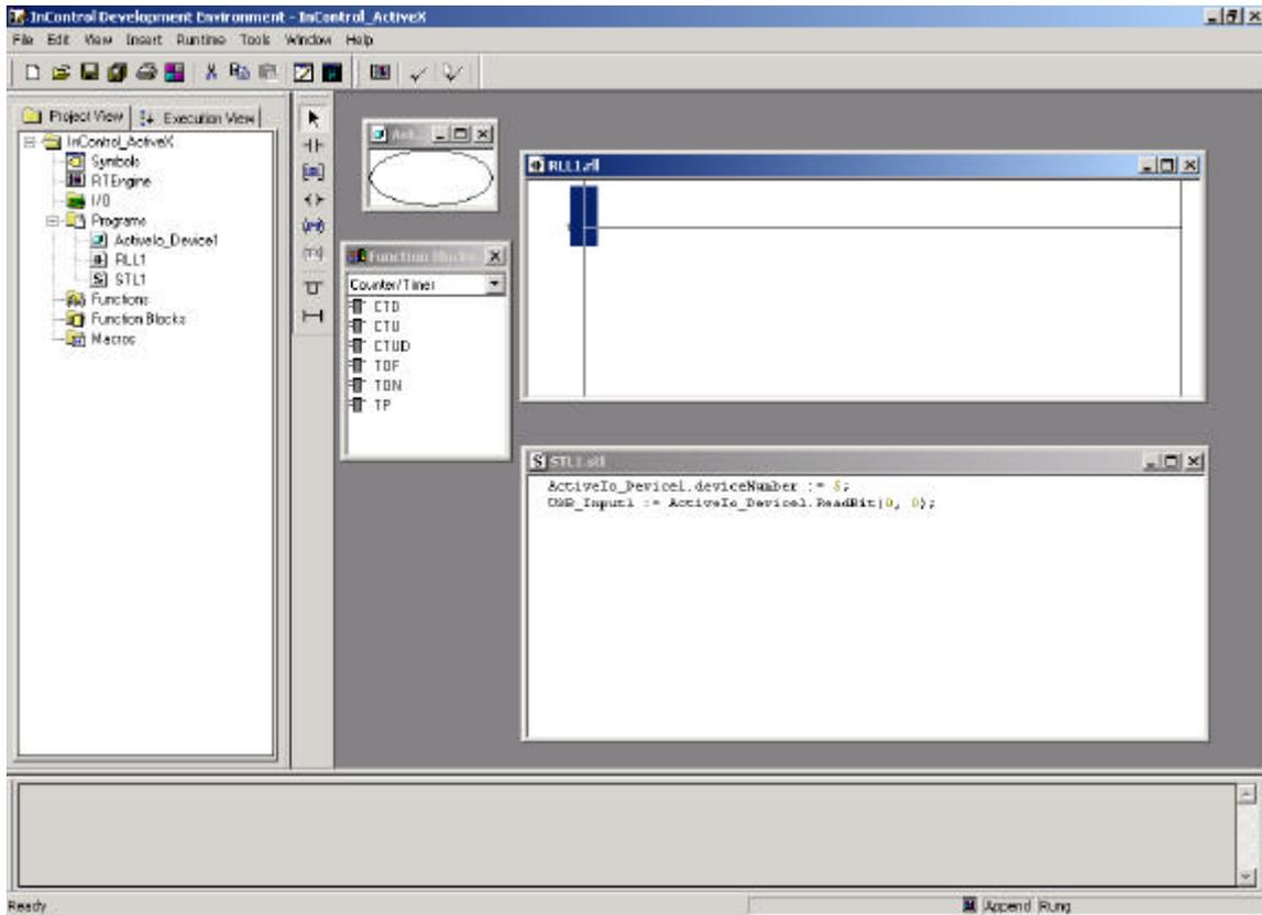
Now we will add a Contact to this rung by using the “Contact Tool” button. Click the “Contact Tool” button and drop the contact on the rung. The following dialog now pops up:
