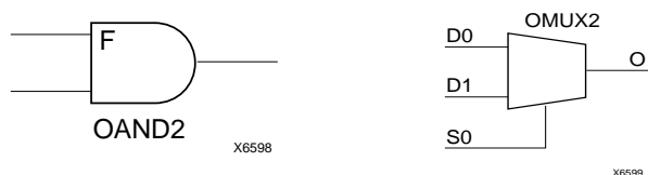
Figure 21: AND & MUX Symbols in XC4000X IOB
