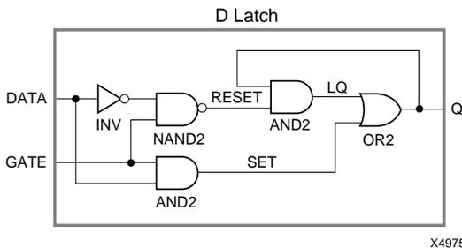
**Figure 2-14 D Latch Implemented with Gates**
