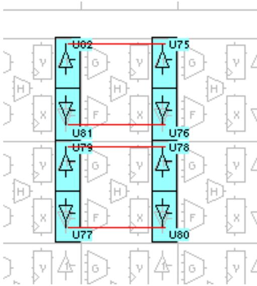
**Figure 4-20** Aligning BUFTs
