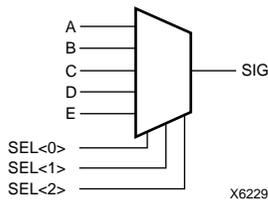
**Figure 3-26 5-to-1 MUX Implemented with Gates**
