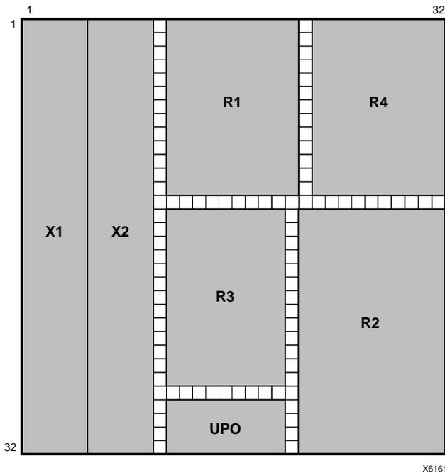
**Figure 6-9 Inefficient Placement of Top Design**
