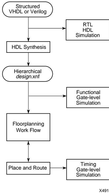
**Figure 1-1 HDL Flow Diagram for a New Design**
