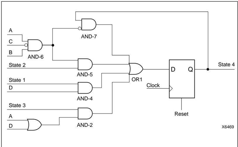
**3. OF THE SEVEN STATES**, the state-transition logic required for State 4 is the most complex, requiring inputs from three other state outputs as well as four of the five condition signals (A - D).
