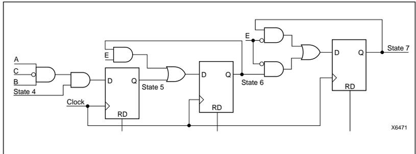
**5. LOOKING NEARLY THE SAME** as a simple shift register, the logic for States 5, 6, and 7 is very simple. This is because the OHE scheme eliminates almost all decoding logic that precedes each flip-flop.
