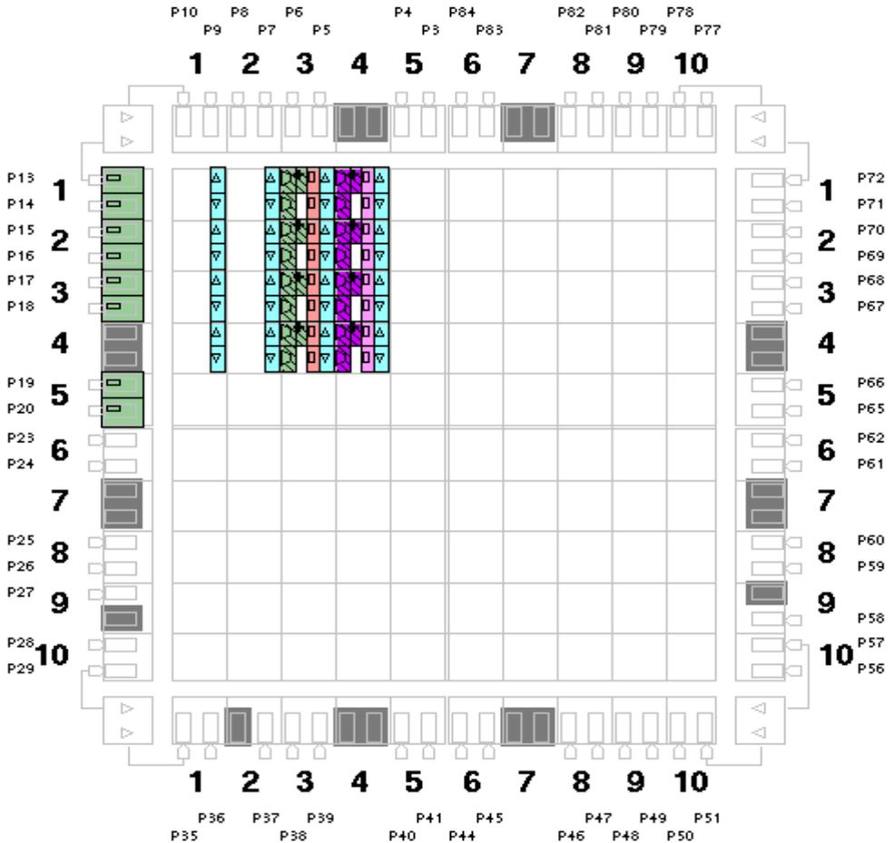
**Figure 4-31 Floorplanned Constraints**
