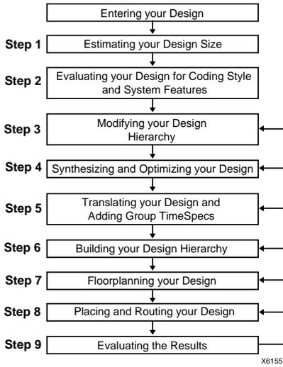
**Figure 6-1 High-Density Design Flow**
