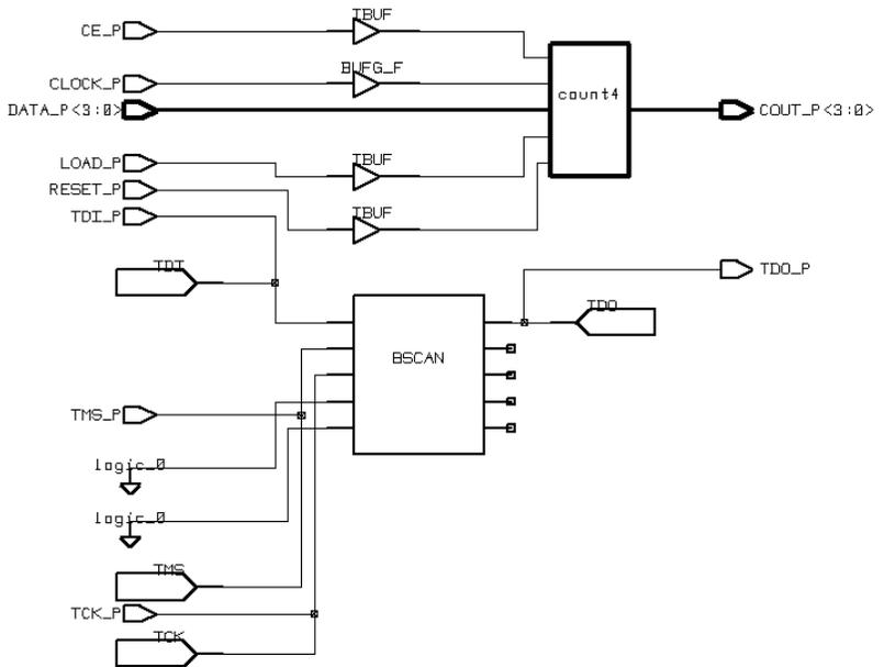
Figure 3-21 Bnd\_scan Schematic
