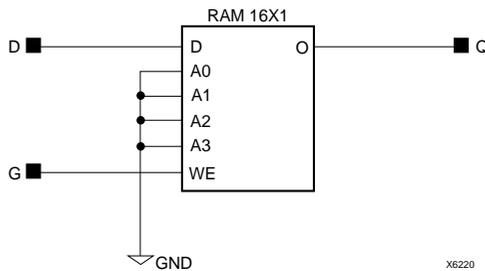
**Figure 2-16 D Latch Implemented by Instantiating a RAM**
