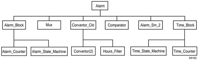
**Figure 4-22 Digital Display Alarm Clock Design Hierarchy**
