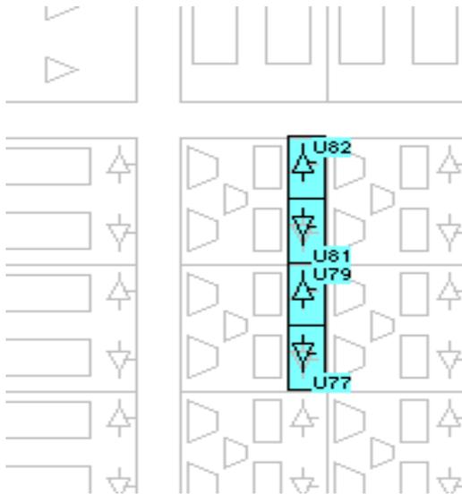
**Figure 4-19 Placing BUFTs in the Floorplan Window**
