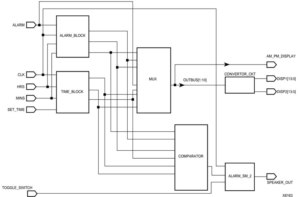
**Figure 4-21 Digital Display Alarm Clock Design**
