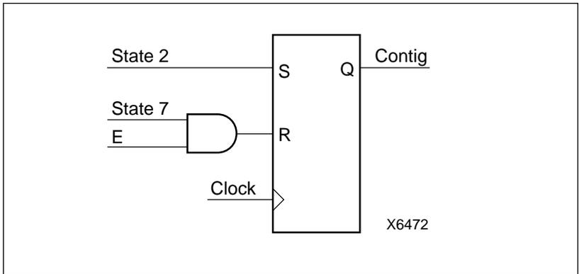
**6. S-R FLIP-FLOPS OFFER ANOTHER** approach to decoding the Contig output. They can also save logic blocks, especially when an output is asserted for a long sequence of contiguous states.
