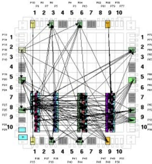
**Figure 4-30 Floorplan Window with Ratsnest Option On**
