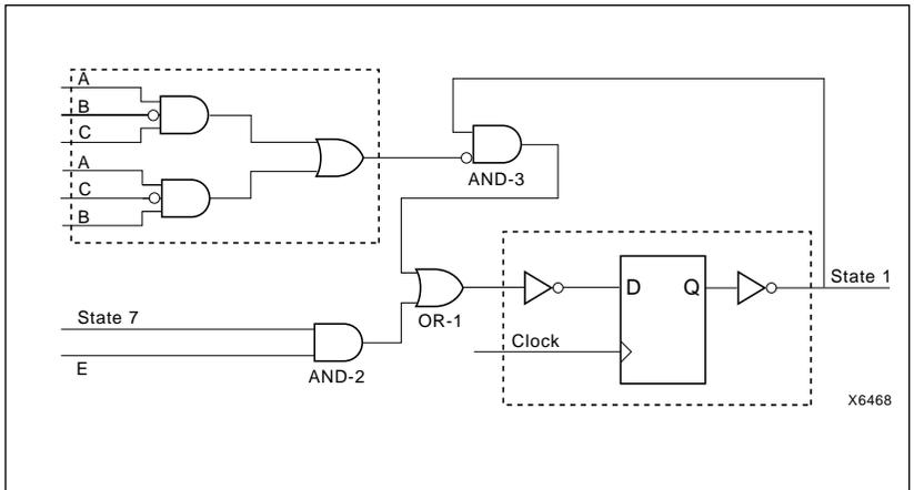
**2. INVERTERS ARE REQUIRED** at the D input and the Q output of the state flip-flop to ensure that it powers on in the proper state. Combinatorial logic decodes the operations based on the input conditions and the state feedback signals. The flip-flop will remain in State 1 as long as the conditional paths out of the states are not valid.
