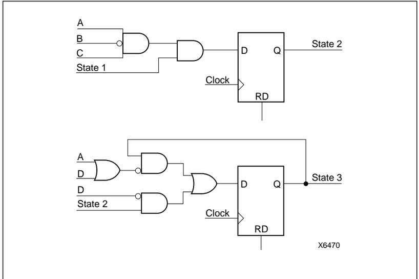
**4. ONLY A FEW GATES** are required by States 2 and 3 to form simple state-transition logic decoding. Just two gates are needed by State 2 (top) , while four simple gates are used by State 3 (bottom).
