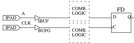
**Figure 5-12 Setup to Clock at the Pad Path**
