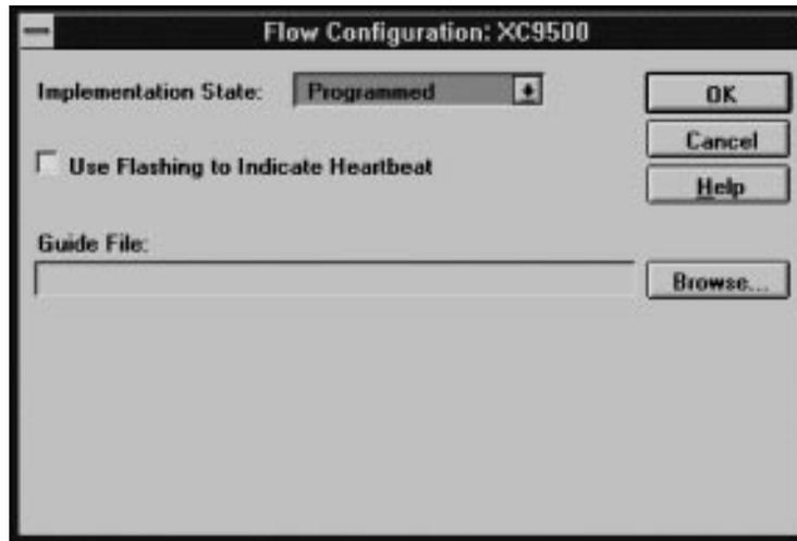
**Figure 2-47 The Flow Configuration Dialog Window**
