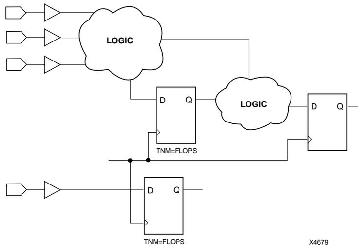
**Figure 4-4 Placing a TNM on Primitive Symbols**
