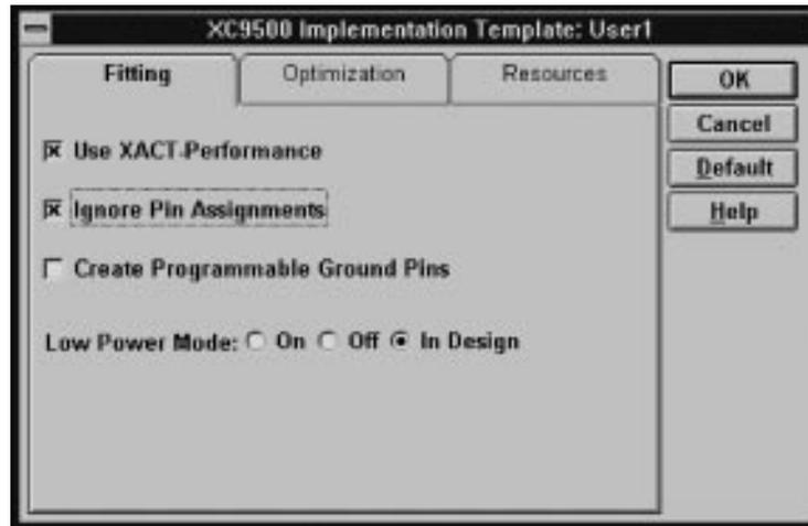
**Figure 2-34 The Fitting Options Template**
