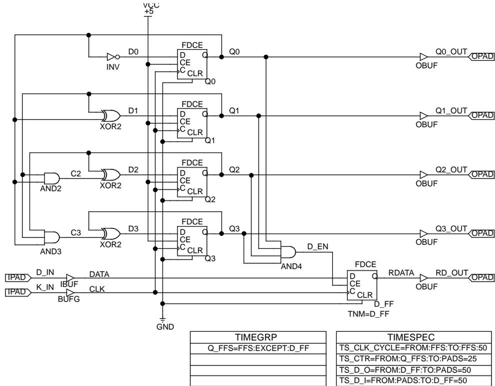
Figure 4-8 Using TNMs and TIMEGRPs in a Schematic
