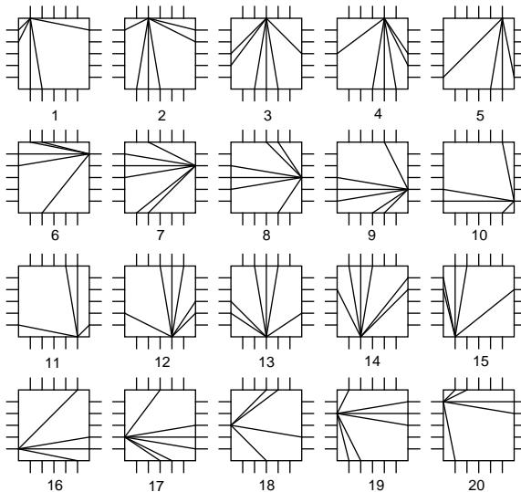
**Figure 9-17 Possible Connections in a Switch Matrix**
