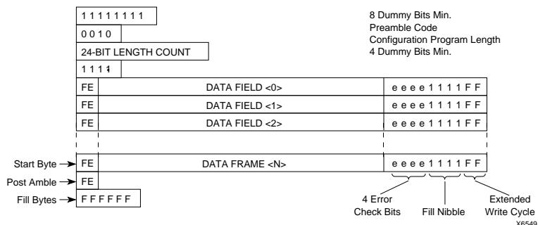
**Figure 7-8 XC5200 Configuration Bitstream Format**
