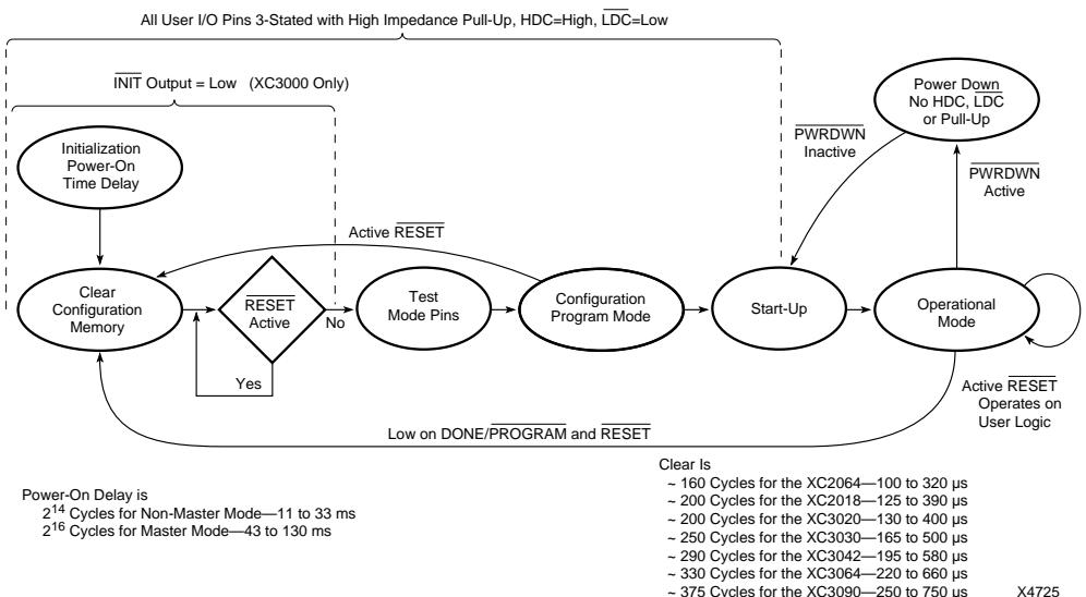
**Figure 6-18 State Diagram for XC2000/XC3000 Devices**
