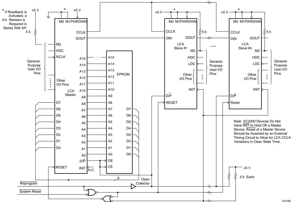
**Figure 6-4 Master Parallel Mode for XC3000/XC3100 Devices**
