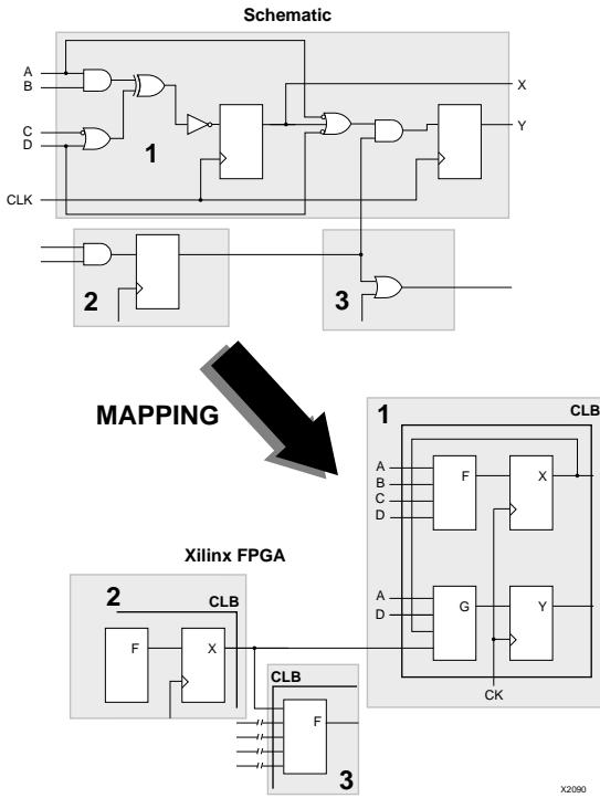
**Figure 3-1 Logic Being Mapped into XC3000 CLBs**
