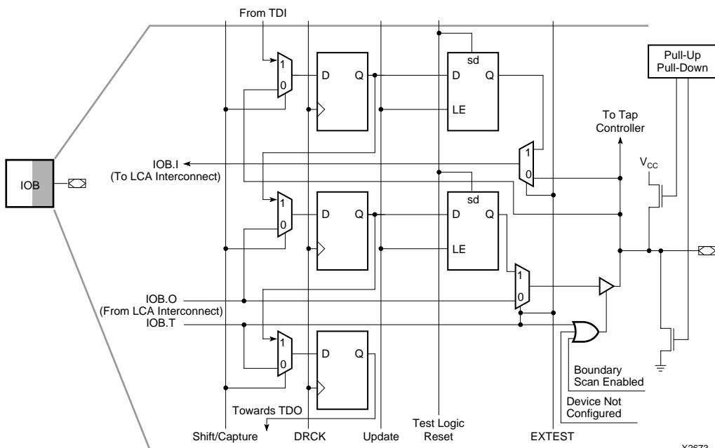
**Figure 8-3 XC4000 and XC5200 Boundary Scan Logic in a TAP Input IOB (TMS, TCK, and TDI Only)**
