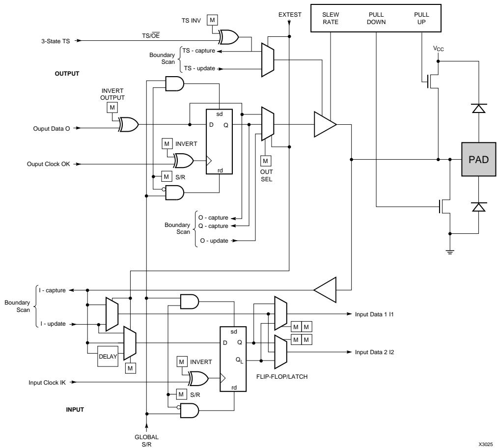
**Figure 1-6 XC4000/XC4000A IOB Structure**
