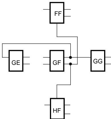
**Figure 1-11 Example of CLBs with Direct Interconnect (XC3000)**
