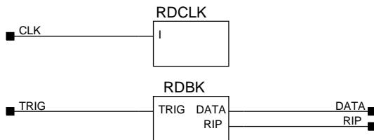
**Figure 7-5 The READBACK Primitive**
