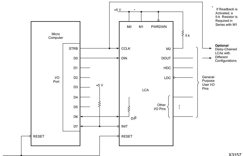
**Figure 6-10 Slave Serial Mode for XC3000/XC3100 Devices**
