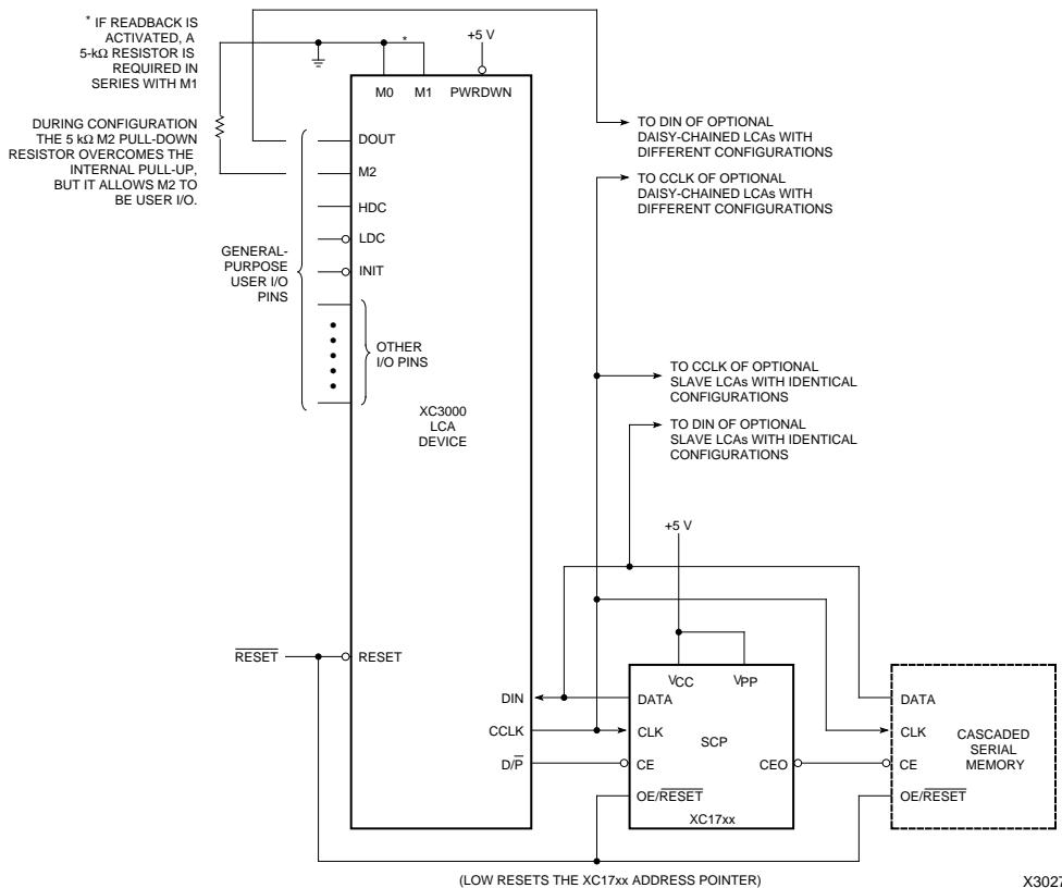
**Figure 6-6 Master Serial Mode for XC3000/XC3100 Devices**
