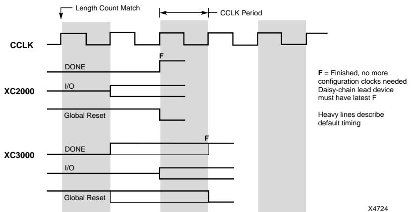
**Figure 6-19 Start-up Timing for XC2000/XC3000 Devices**
