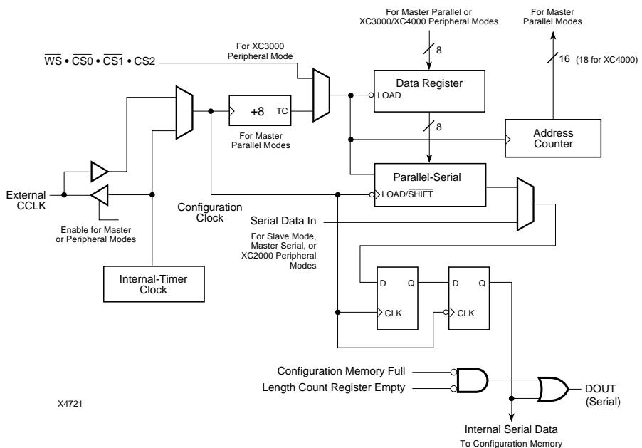
**Figure 6-16 Mode-Line Logic Level Inputs to the FPGA Control Configuration Data Path Multiplexers**
