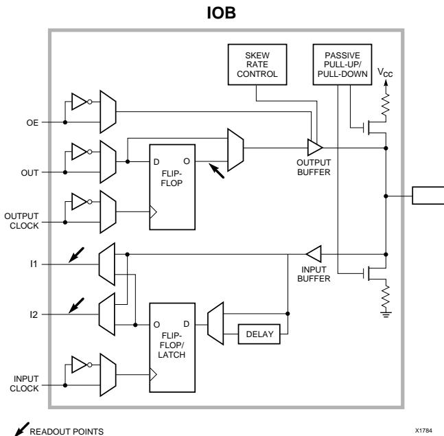
**Figure 7-1 XC4000 IOB Logic Configuration**
