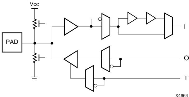
**Figure 1-5 XC5200 IOB Structure**
