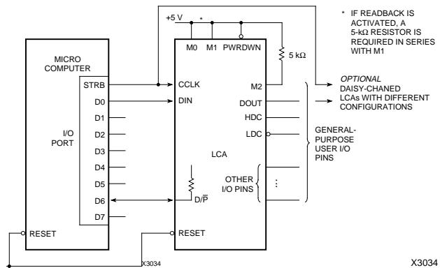
**Figure 6-9 Slave Serial Mode for XC2000 Devices**
