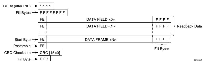
**Figure 7-10 XC5200 Readback Bitstream**
