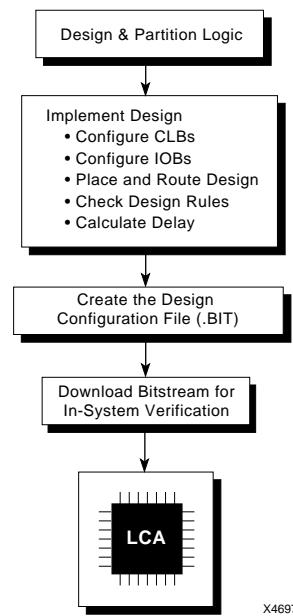
**Figure 9-26 FPGA Design Flow Using XDE**
