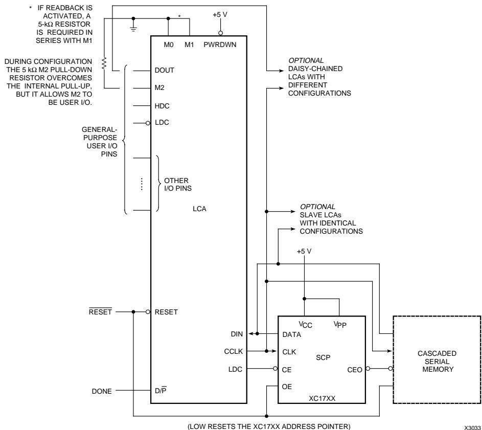
**Figure 6-5 Master Serial Mode for XC2000 Devices**
