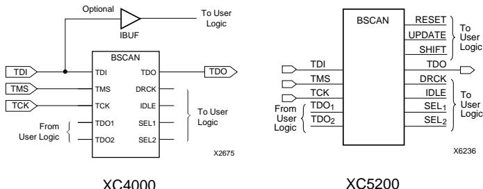
**Figure 8-6 Boundary-Scan Schematic Symbols for XC4000 and XC5200**
