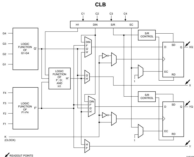
Figure 7-2 XC4000 CLB Logic Configuration
