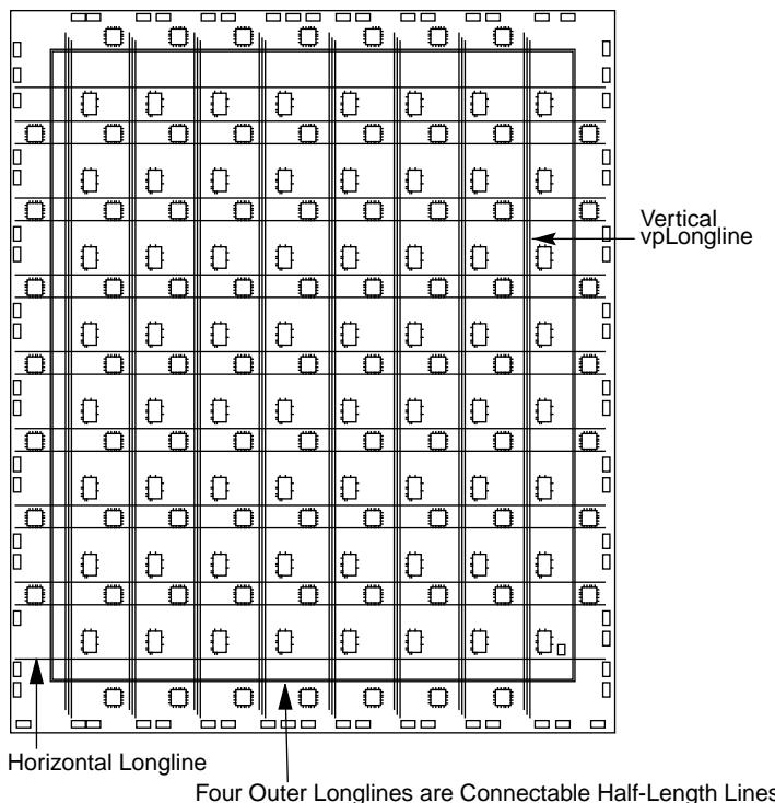
**Figure 1-10 Horizontal and Vertical Longlines (XC3000)**
