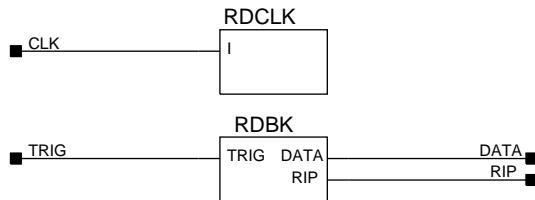
**Figure 7-6 READBACK Symbol on the Schematic**
