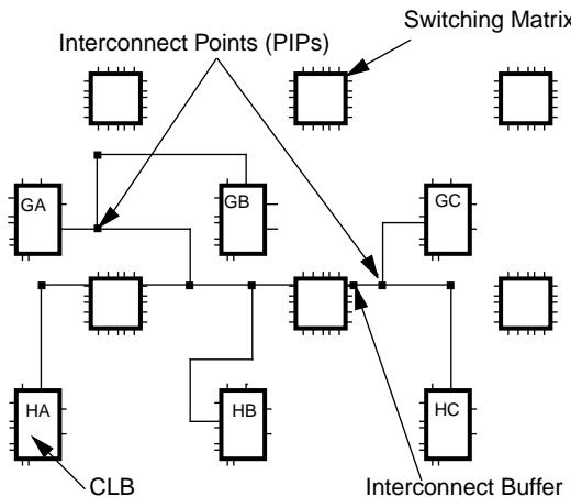
**Figure 1-13 Programmable Interconnect Points (PIPs)**
