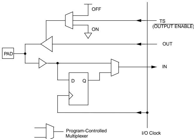
**Figure 1-9 XC2000 IOB Structure**
