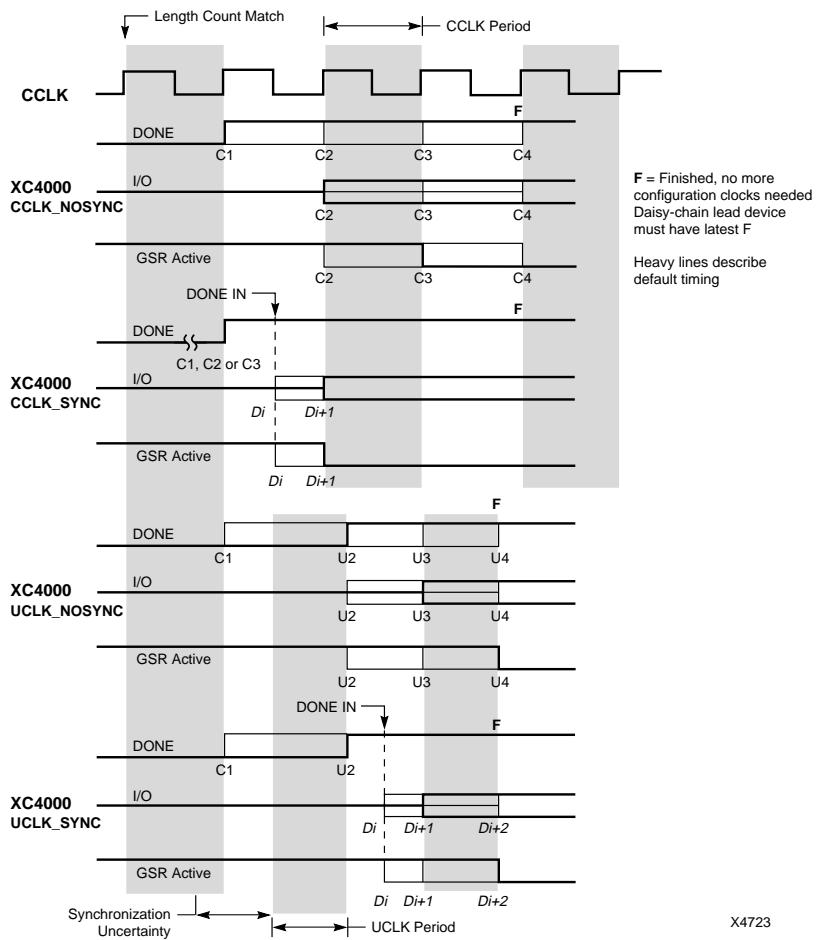
**Figure 6-21 Start-up Timing for XC4000/XC5200 Devices**
