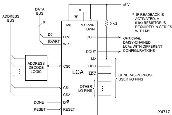
**Figure 6-7 Peripheral Mode for XC2000 Devices**
