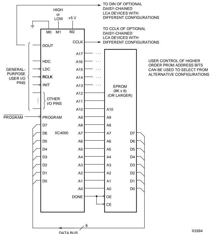
**Figure 6-11 Master Parallel Mode for XC4000 and XC5200 Devices**
