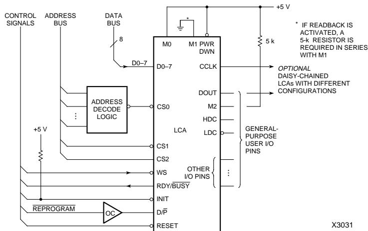
**Figure 6-8 Peripheral Mode for XC3000/XC3100 Devices**
