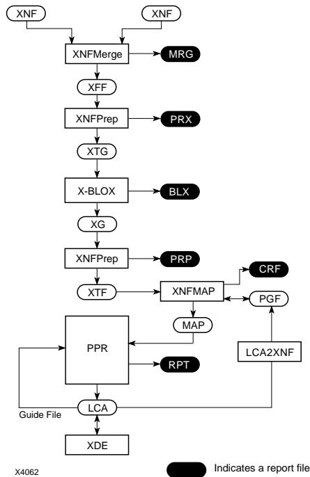
**Figure 5-2 XC3000A/XC3000L/XC3100A Design Flow**
