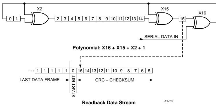
**Figure 7-13 Circuit for Generating the CRC-16**
