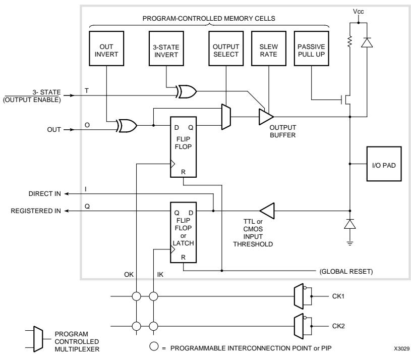
**Figure 1-8 XC3000 IOB Structure**
