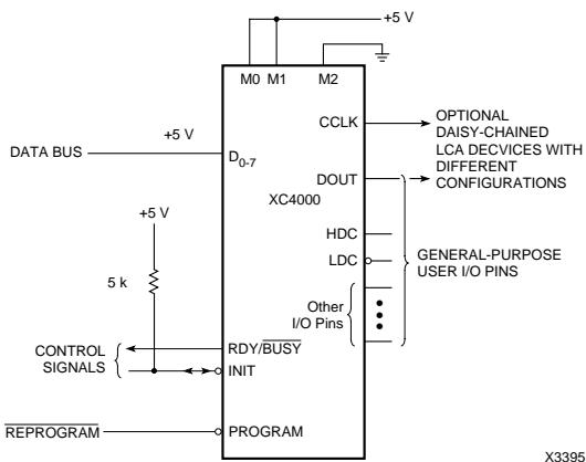
**Figure 6-13 Synchronous Peripheral Mode for XC4000 and XC5200 Devices**
