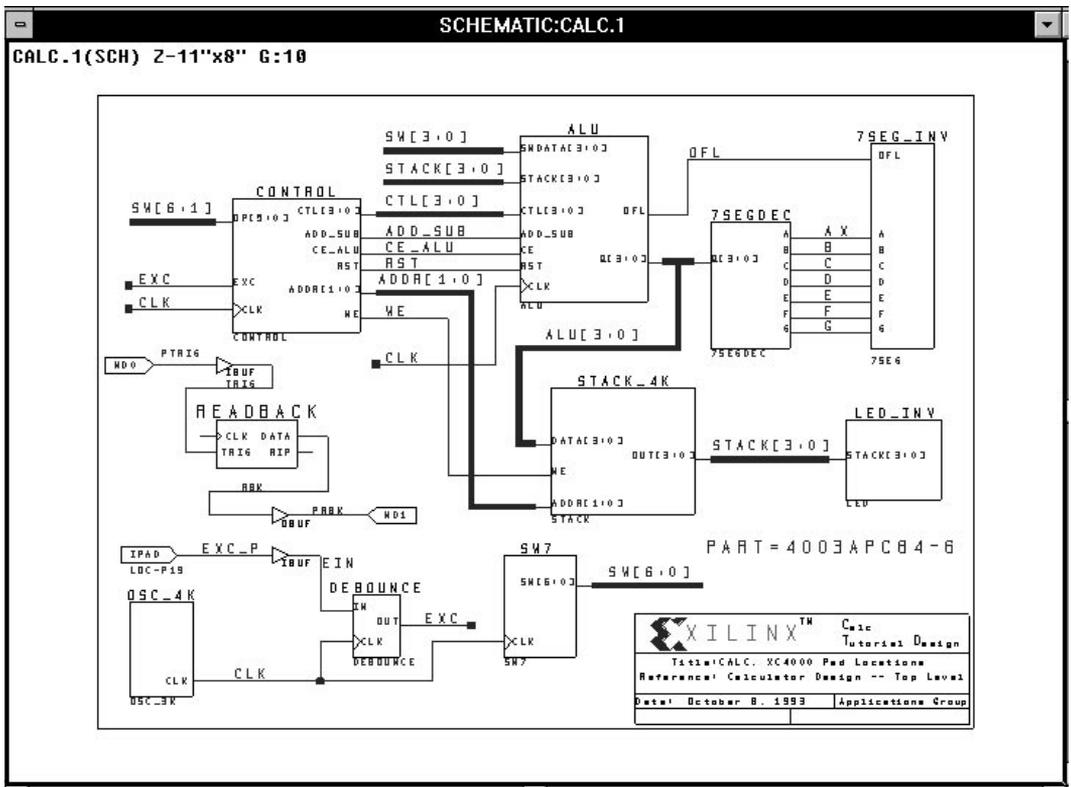
Figure 10-1 Calc Schematic
