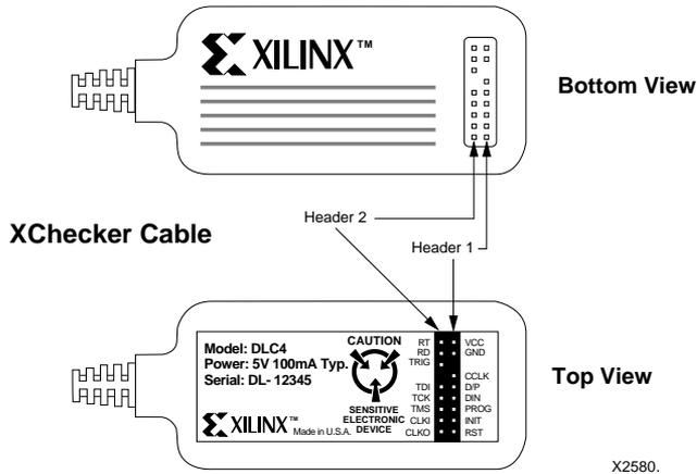
**Figure 4-2 XChecker Cable Pins**
