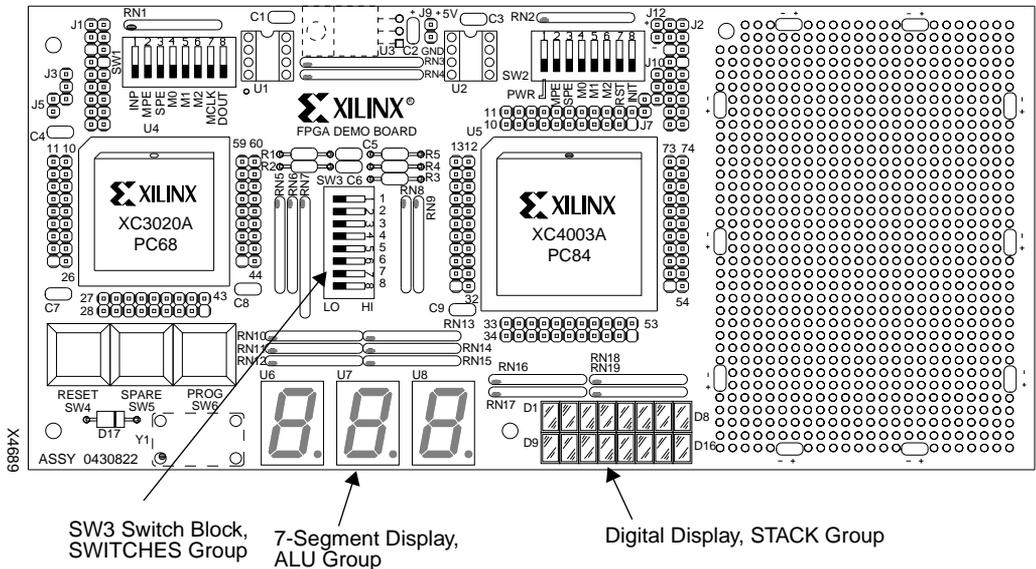
Figure 10-14 FPGA Demonstration Board Components
