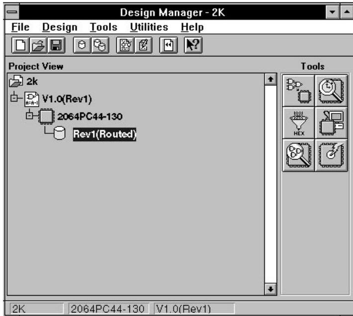
**Figure 3-4 Routed XC2000 Design in the Design Manager**
