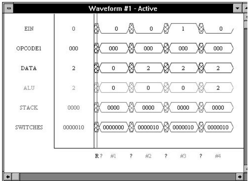
**Figure 10-15 Capturing the Device States for the Add Operation**
