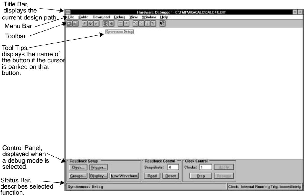
**Figure 2-2 Hardware Debugger Main Window**
