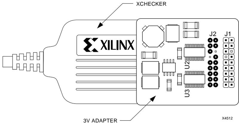
**Figure A-2 XChecker 3-Volt Adapter**
