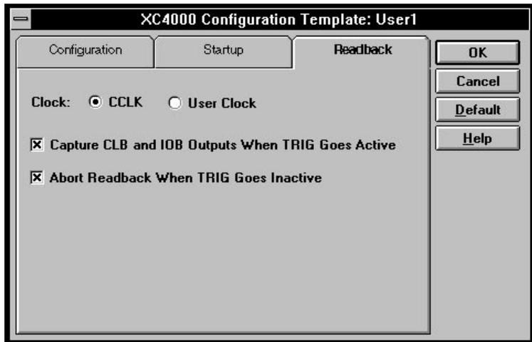
**Figure 10-6 Design Manager Readback Data Screen**
