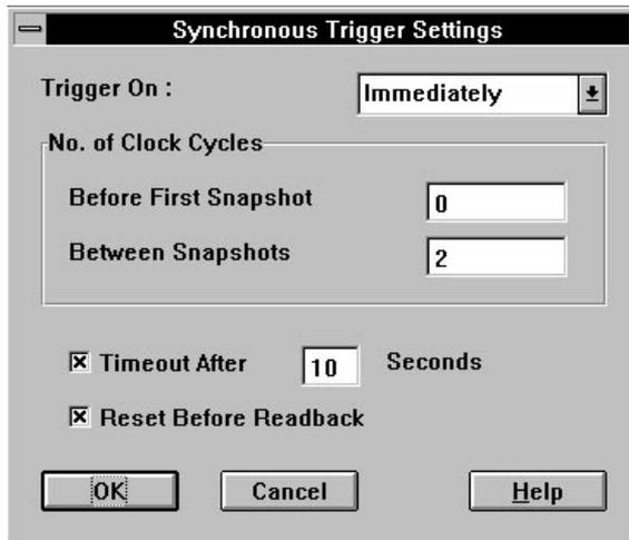
**Figure 6-4 Synchronous Trigger Dialog Box**
