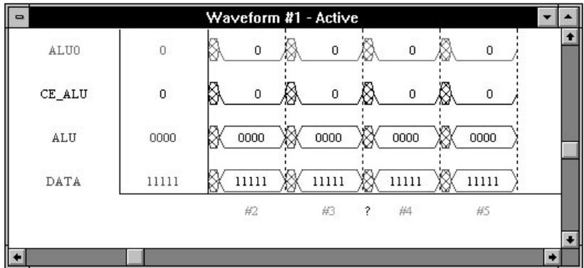
**Figure 7-7 The Active Waveform Window (Graphical View)**
