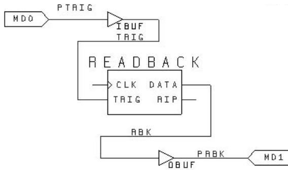
**Figure 10-2 Readback Symbol Connections**
