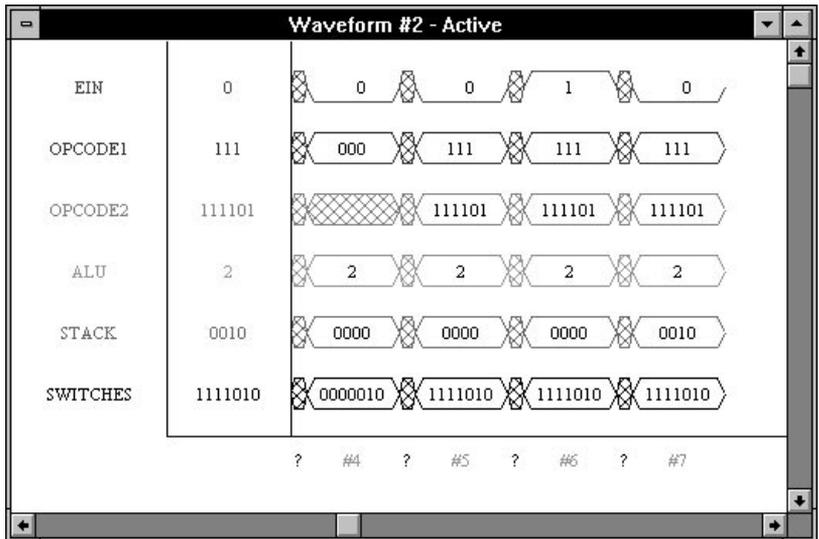
**Figure 10-18 Capturing the Device States for the Push Operation**
