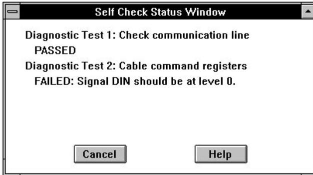
**Figure 8-30 Failed Self-Check Test**
