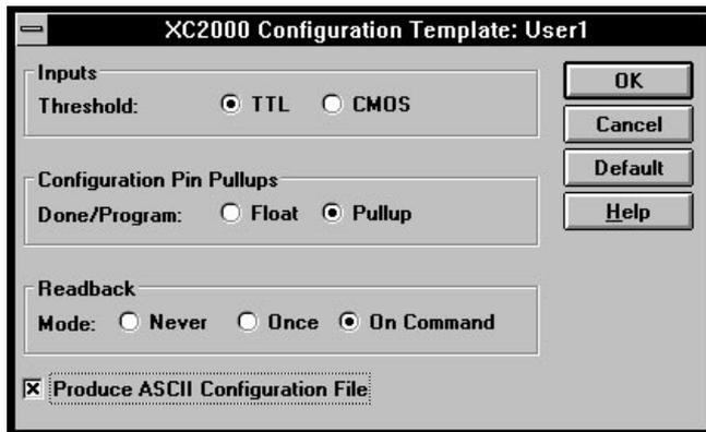
Figure 3-6 Design Manager Configuration Dialog Box (XC2000)
