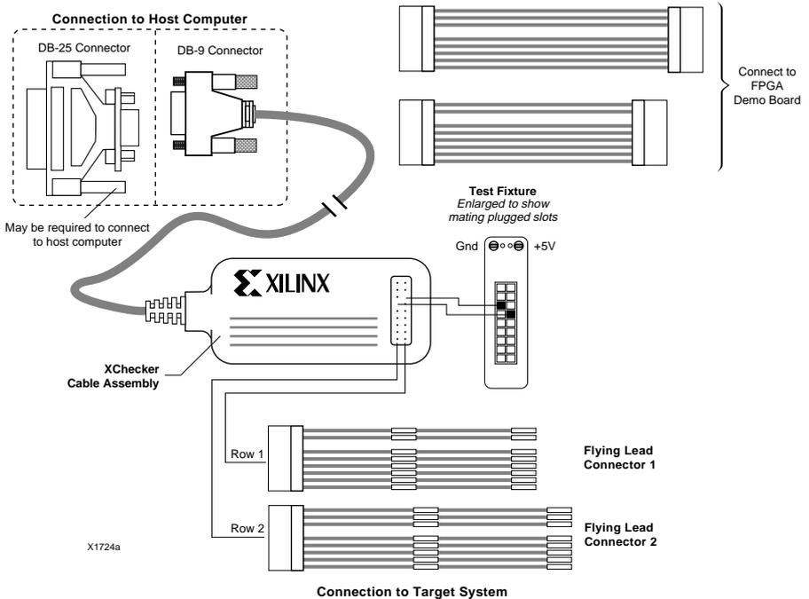
**Figure 4-1 XChecker Cable with Connectors and Test Fixture**
