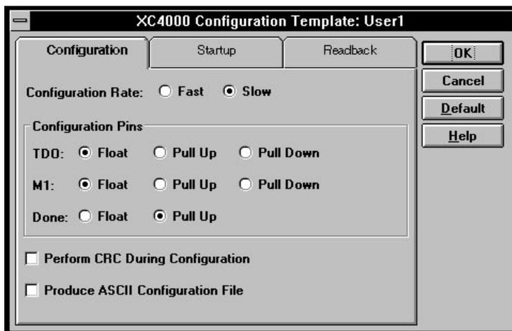
**Figure 3-10 Design Manager Configuration Template**
