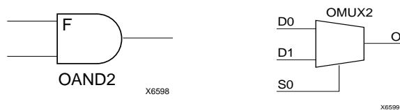
Figure 7: AND & MUX Symbols in SpartanXL IOB
