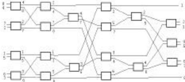
Figure 3: Sorting network for sequence of size eight.
