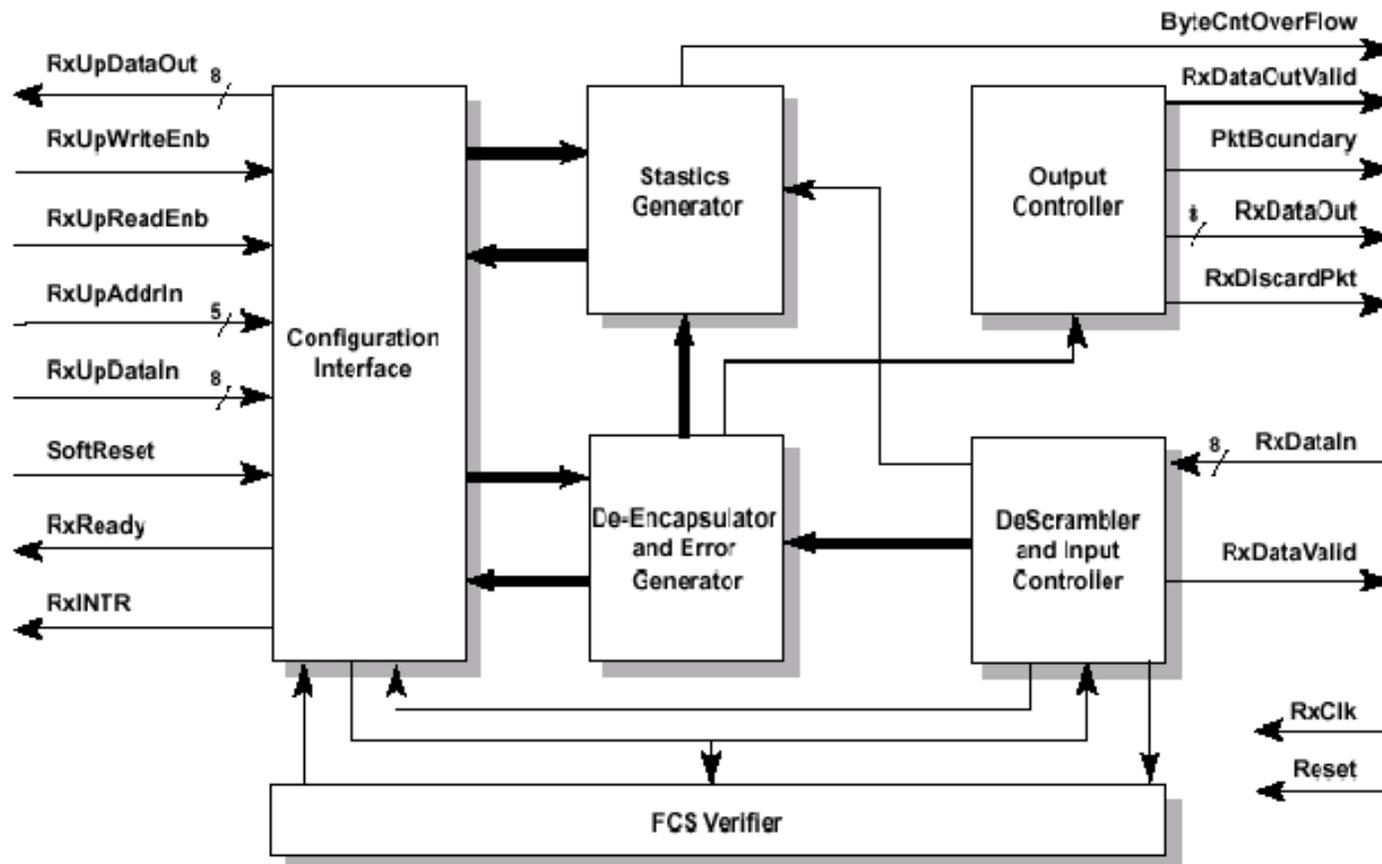
CC318f HDLC Controller (Receiver) Block Diagram
