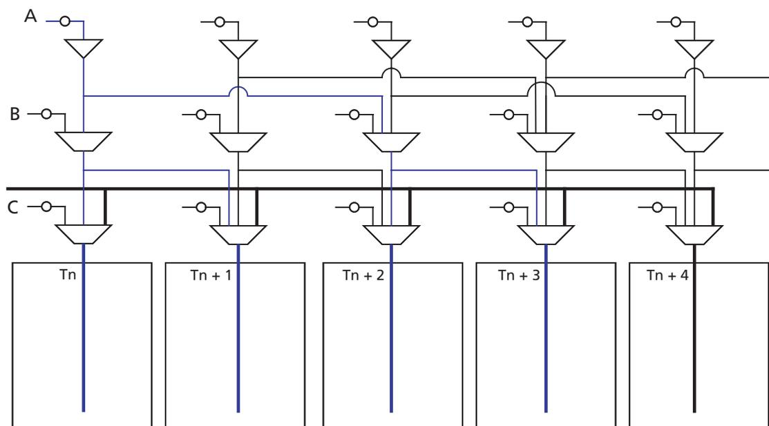
Figure 4 • Four Spines Aggregation
