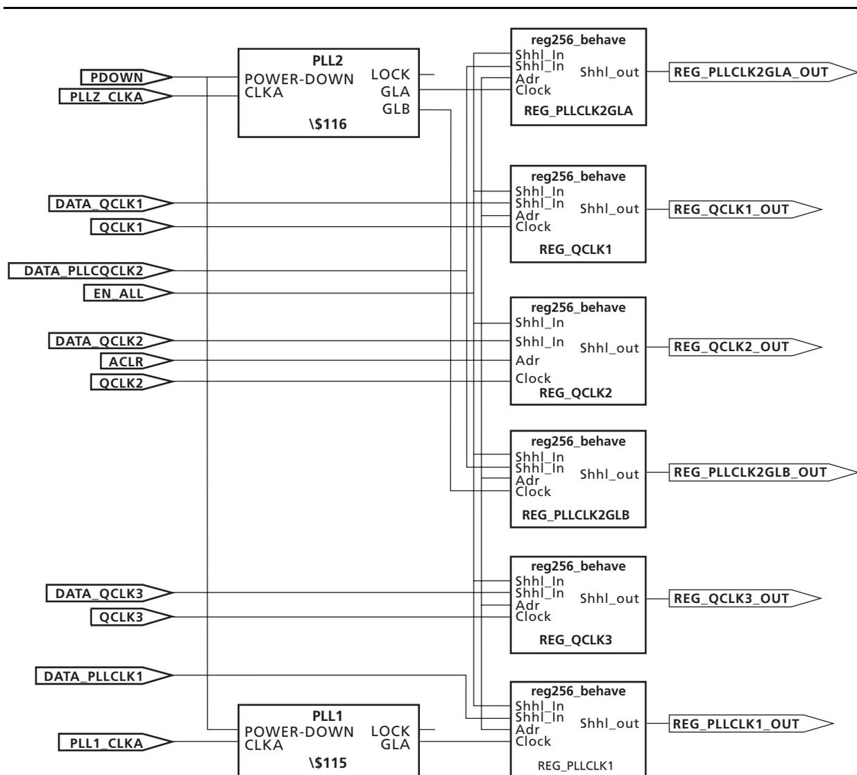
Figure 10 • Block Diagram of the Global Management Example Design
