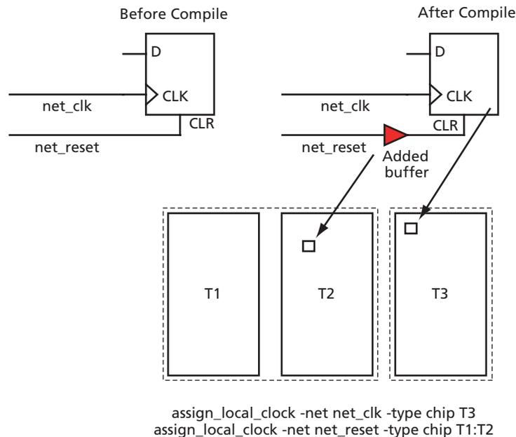
Figure 7 • Adding a Buffer for Shared Instances
