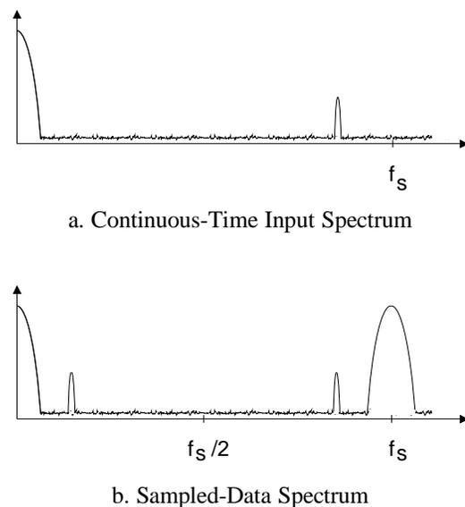
**Figure 6. Sampled-Data Spectrum**
