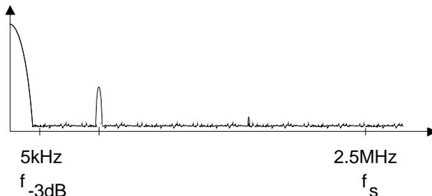
b. Modulator Digital Output Spectrum
