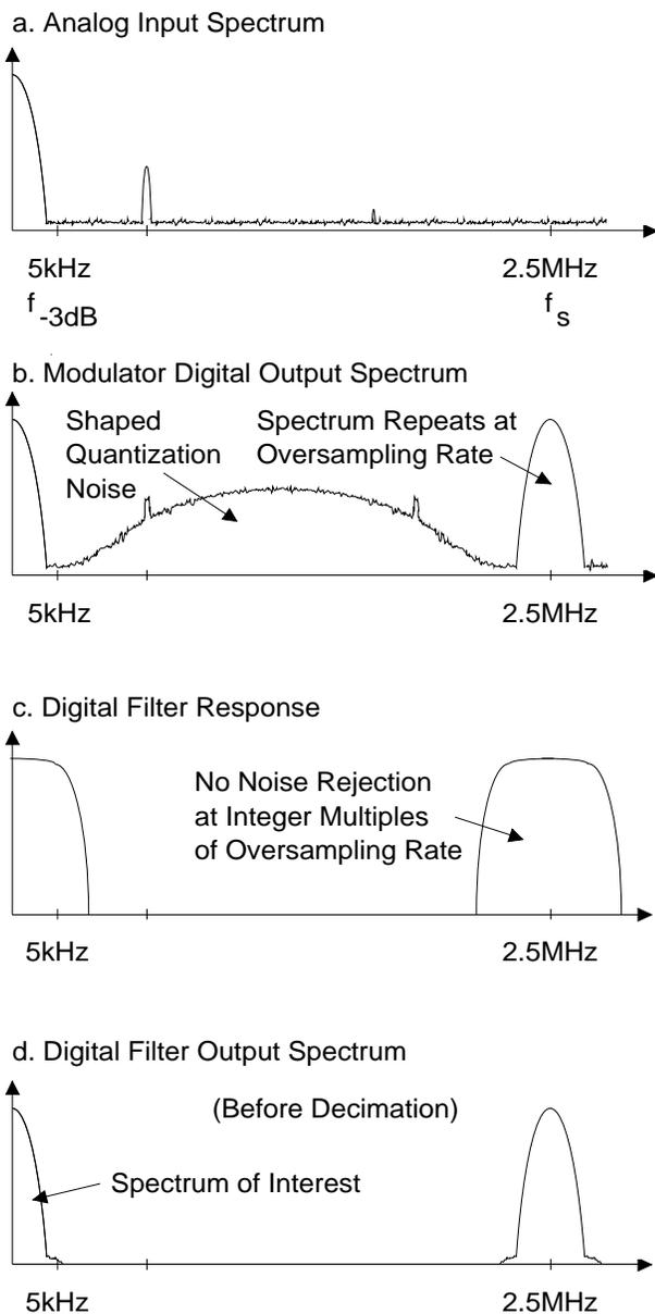
**Figure 4. Delta-Sigma Spectral Analysis**
