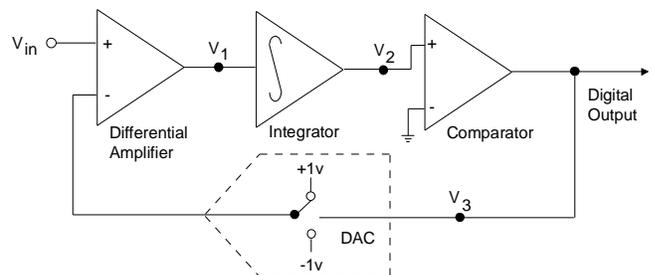
**Figure 2. 1<sup>st</sup>-order Delta-Sigma Modulator**
