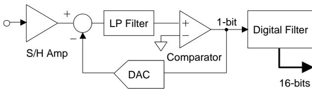
**Figure 1. Delta-Sigma ADC**
