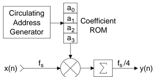
**Figure 9. 4<sup>th</sup>-order FIR Filter with 4X Decimation**
