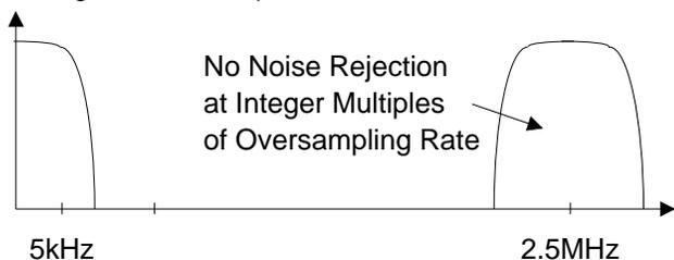
d. Digital Filter Output Spectrum
