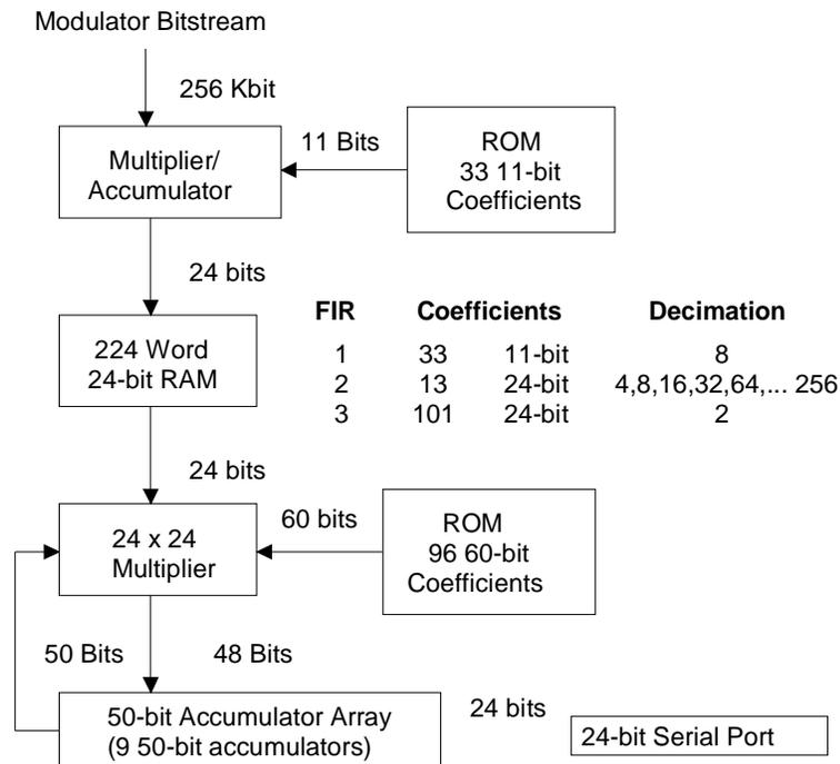
Figure 1. Digital Filter Block Diagram
