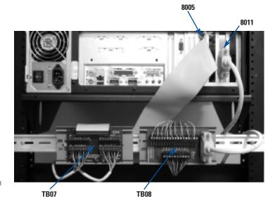
alarm system just to name a few. Conversely, optically isolated inputs are used to convert incoming control signals to electrical levels that are compatible with the host computer. Optical isolation is often used to protect the PC from voltage spikes or over-current situations.
