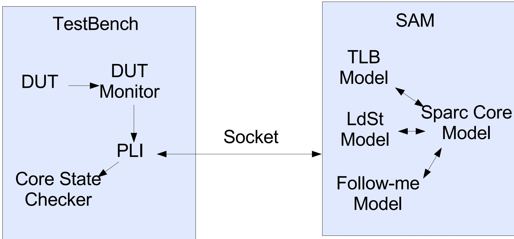
\* DUT: device under test, i.e., RTL
