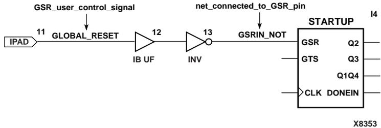
Figure 5-7 Verilog User-Controlled Inverted GSR
