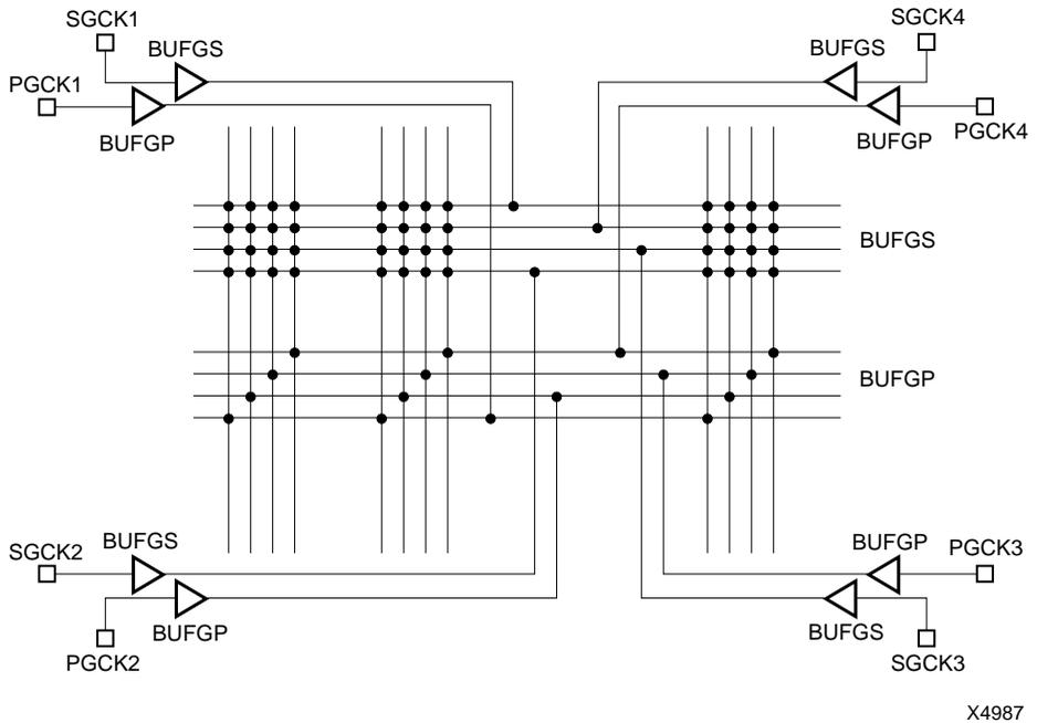
**Figure 4-1 Global Buffer Routing Resources (XC4000E, Spartan)**
