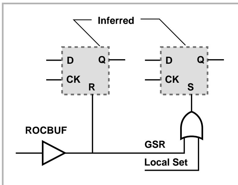
**Figure 5-4** ROCBUF Simulation and Implementation
