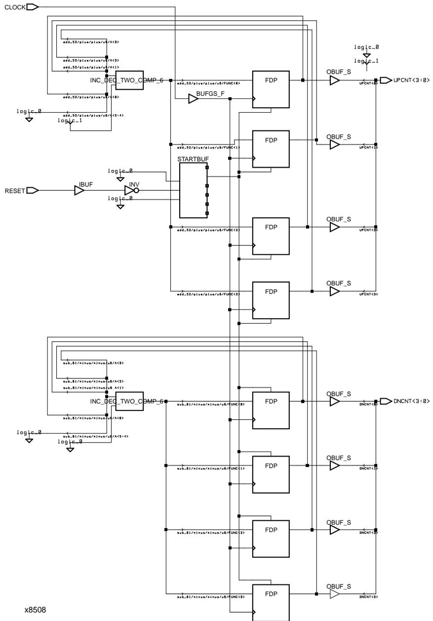
Figure 4-5 Use\_GSR Implemented with Gates
