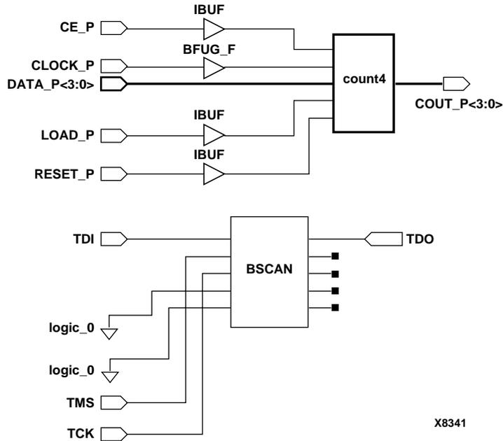
Figure 4-8 Bnd\_scan Schematic
