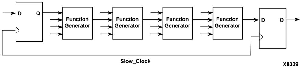
Figure 4-12 Before Pipelining
