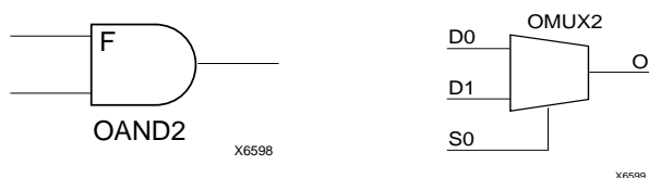
Figure 7: AND & MUX Symbols in Spartan-XL IOB
