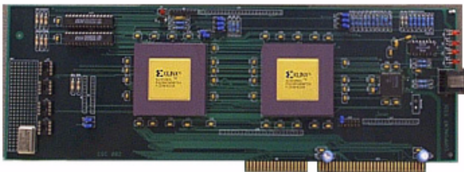
Figure 1: 10/100 Ethernet NIC Board
