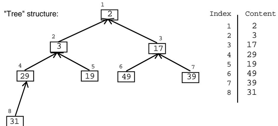
Figure 21.2 "Tree" of partially ordered values and their mapping into an array.
